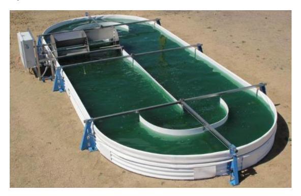
Figure 9 – Microalgae Raceway Pond
