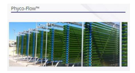
Figure 10 – Microalgae Photobioreactor
