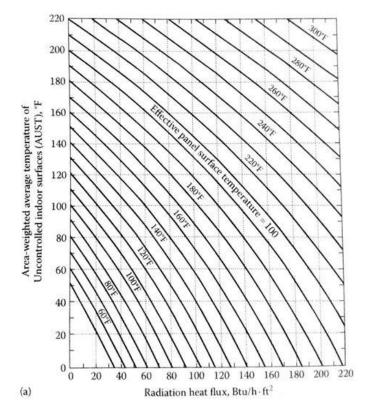
Figure 19: Radiation heat flux plots for ceiling, wall or floor heated panels
