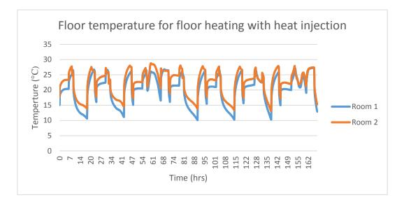
Figure 33: Floor heating with heat injection zone floor temperature
