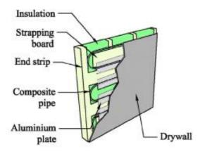
Figure 21: Wall or ceiling heating panel
