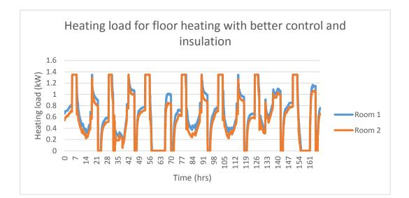
Figure 37: Floor heating with better control and insulation heating load
