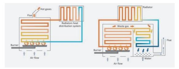
Figure 13: Traditional (left) and condensing boiler (right) flow system
