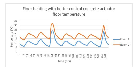
Figure 64: Floor temperature for floor heating with better control and concrete
