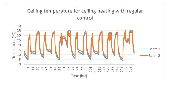
Figure 40: Ceiling heating with regular control ceiling temperature
