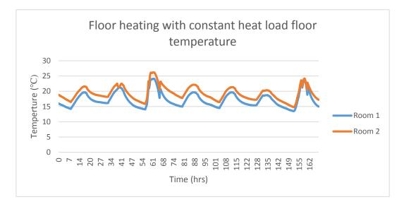
Figure 65: Floor temperature for floor heating with constant 600W heat input
