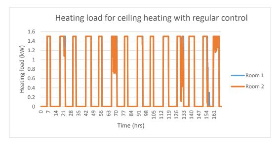
Figure 41: Ceiling heating with regular control heating load
