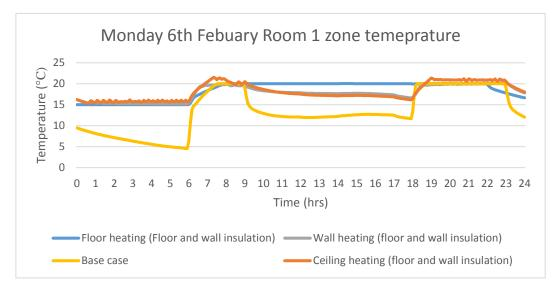
Figure 53: Best floor, ceiling and wall heating configuration using original simulation method
