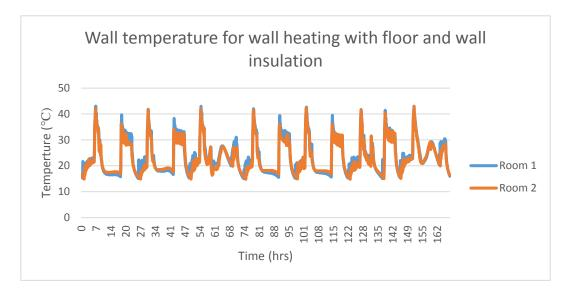
Figure 49: Wall heating with floor and wall insulation wall temperature
