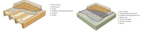
Figure 17: Timber floor UFH design with lightweight screed
