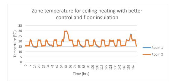
*Figure 42: Ceiling heating with better control and floor insulation zone temperature*
