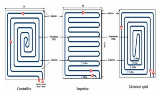
Figure 59: Three possible pipe configurations for UFH (Oubenmoh et al., 2018)
