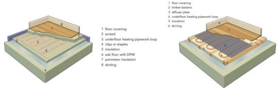
Figure 15: Concrete floor UFH design
