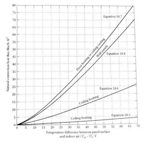
Figure 20: Natural convective heat transfer for floor, ceiling and wall panels
