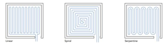
Figure 18: Typical UFH pipework layout patterns
