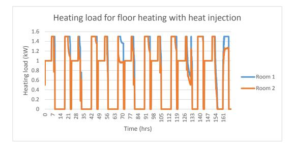
Figure 34: Floor heating with heat injection heating load
