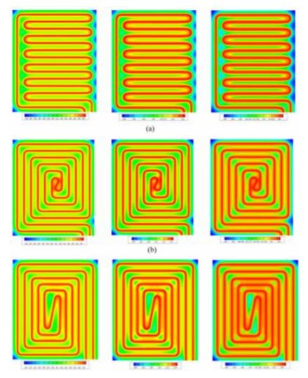
Figure 60: Floor surface temperature of three configuration from 35-50°C left to right (Oubenmoh et al., 2018)
