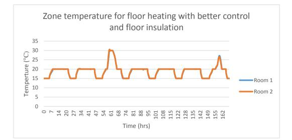
Figure 35: Floor heating with better control and floor insulation zone temperature
