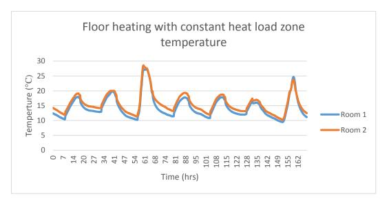
Figure 66: Zone temperature for floor heating with constant 600W heat input
