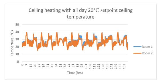
*Figure 71: Ceiling temperature for ceiling heating with better control 20°C set point*
