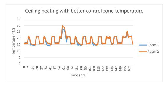
*Figure 68: Zone temperature for ceiling heating with better control no floor insulation*
