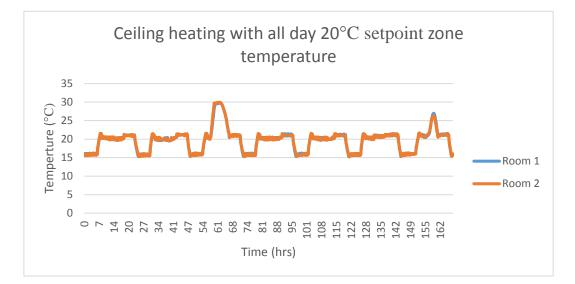
Figure 70: Zone temperature for ceiling heating with better control 20°C set point
