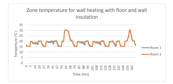
Figure 48: Wall heating with better control and floor+wall insulation zone temperature
