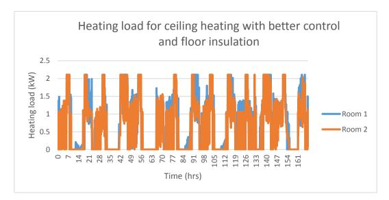
Figure 44: Ceiling heating with better control and floor insulation heating load
