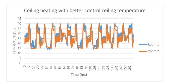
Figure 67: Ceiling temperature for ceiling heating with better control no floor insulation
