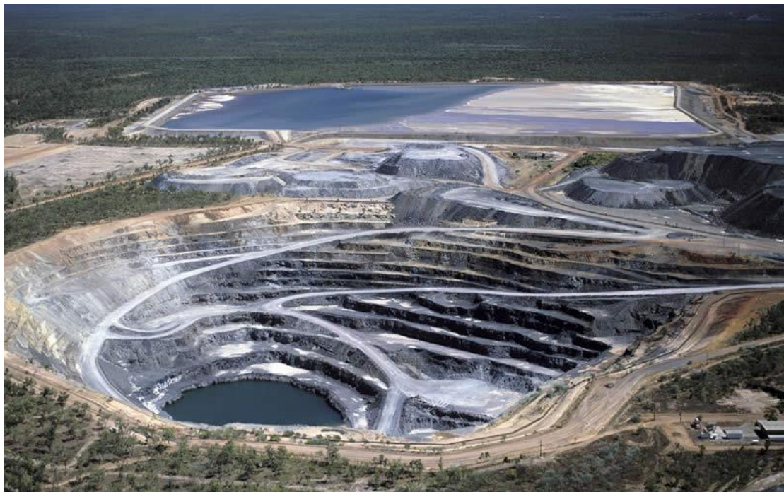
Figure 21: This show one of the conventional methods of mining uranium, also known as open cut mining
