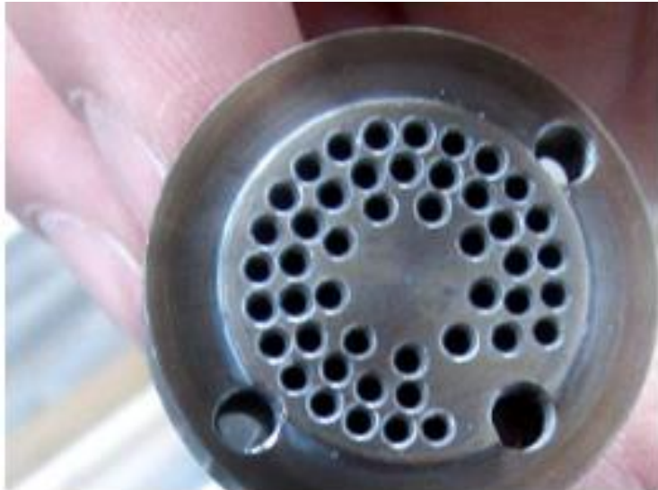
Figure 20: Holes at the top of the rig for sensors to be put through and allows for continuous collection of data from the reactor at OECD
