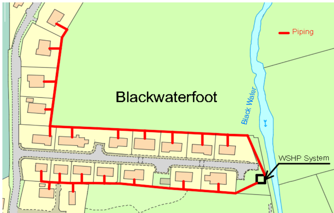
Figure 50. Heat distribution network design of the proposed development sketched in AutoCAD
