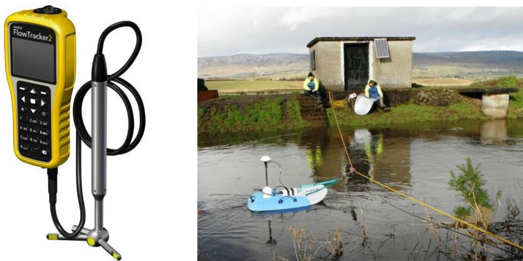
Figure 30. Gauging devices used by hydrologists; Basic Flow Tracker (left) (SonTek, 2017) and advanced cableways device (right) (SEPA, 2017)
