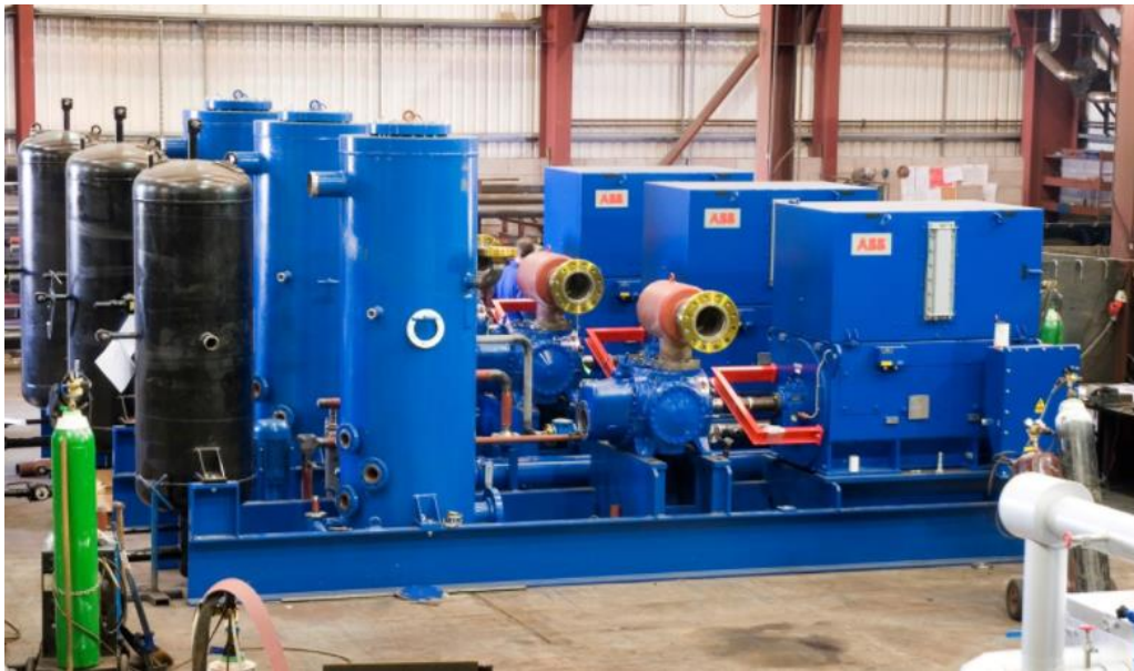
Figure 11. Large-scale river source heat pump with an open-loop system manufactured by Star Renewable Energy (Star Refrigeration, 2016)
