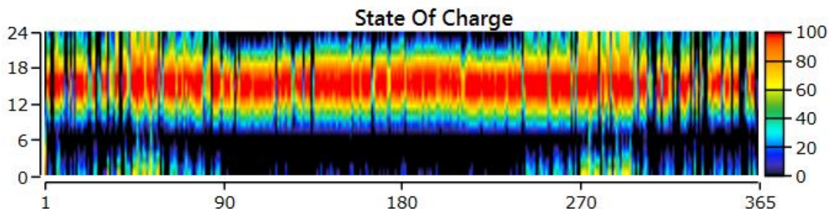
Figure 88: SOC for Gildemeister 250kW-4hr CELLCUBE® FB 250-1000
