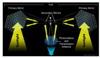
Figure 7- Diagram showing the most common design for SPS systems (National Space Society, 2016)
