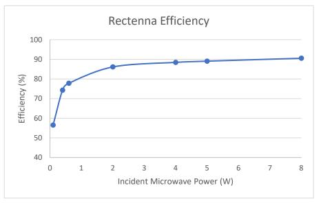
Figure 9 - Graph showing the trend in efficiency of rectennae with low input power
