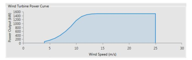
Figure 18 - wind turbine power curve
