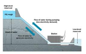
Figure 8- pumped hydro system
