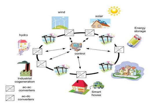
Figure 4:Scheme of a microgrid (compliance,2017)
