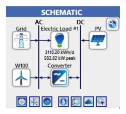
Figure 47: Configuration of the energy system of Capileira with 100 kW of PV capacity plus four turbines WES100
