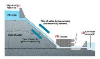
Figure 11: Hydro Pump Storage Operating System (American Society of Civil Engineers, 1996)
