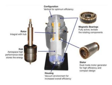
Figure 9: Representation of the components of a Flywheel (Oberhofer, 2012)
