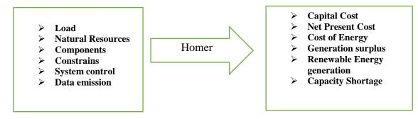
Figure 27: Schematic representation of the functions of HOMER (Sinha and Chandel, 2014)
