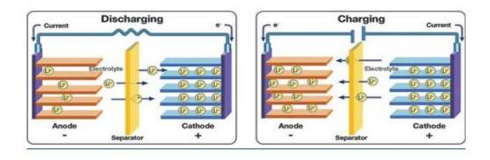
Figure 12: Representation of the operation of a Lithium-ion battery (Research & Development, 2017)
