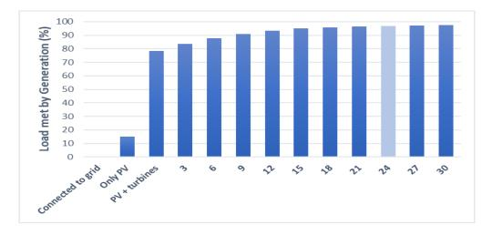
Figure 64: Variation of load met by generation depending of capacity of generation and numbers of RedT 15-75
