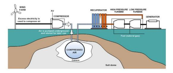
Figure 10: Possible configuration of a CAES system (Sc.ehu.es, 2017)
