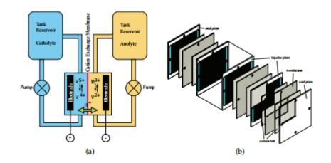
Figure 13: Representation of the performance of a vanadium flow battery (Blanc and Rufer, 2010)
