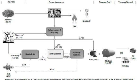
Figure 6: An example of a CO<sub>2</sub>-electrofuel production process: carbon that is sequestered using CCR at a power plant and afterwards, it is hydrogenated to produce methane [42, 76].
