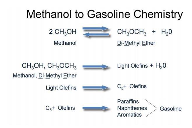
The first stage in the process is the conversion of methanol to di-methyl ether through dehydration. Following this, the DME, and methanol reacts to produce light olefins. Polymerization and hydrogenation stages allow for these olefins to be converted into gasoline, a mixture of paraffins, napthalenes, and aromatics.
