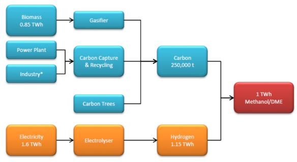
Figure 8: Carbon and hydrogen required to produce electrofuel in the form of methanol or dimethyl ether (DME). A variety of different carbon options are displayed here to illustrate the options available. \*Cement production is one very good example of an industrial process with surplus carbon.
