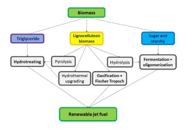
Figure 7 -Synthetic Jet Fuel Production Pathway from Biomass
