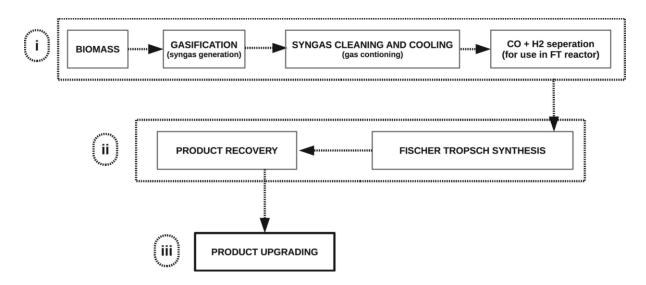
Figure 6 - Biomass to Synthetic Fuels Process
