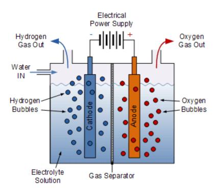
A basic diagram showing water electrolysis is given below: <sup>25</sup>
