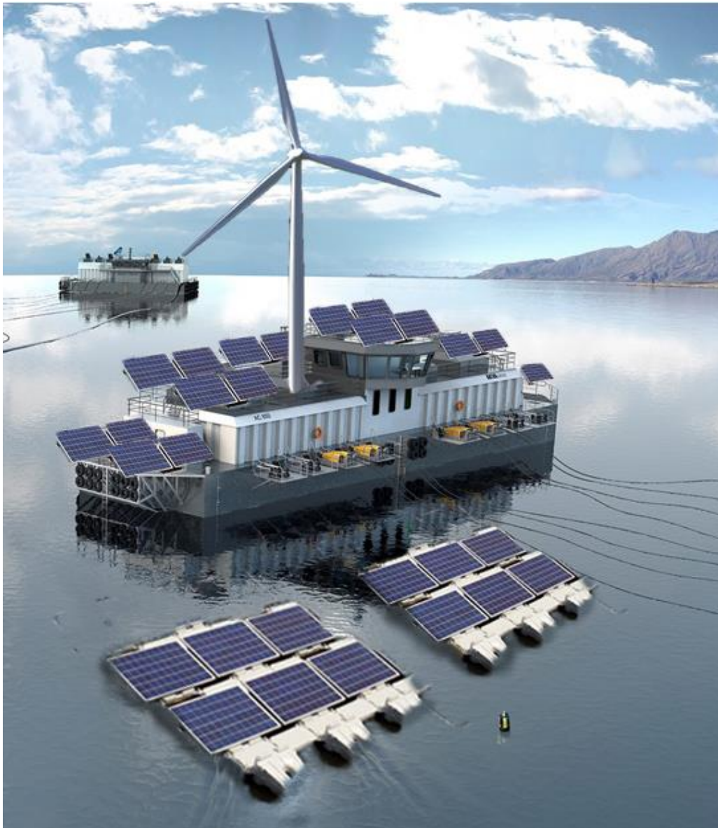
Figure 39 The feed barge with the cost optimal hybrid system . The wind turbine has a capacity of 14 kW, and there is a total of 35 kW of PV capacity. Below deck there are Li-Ion batteries with a total capacity of 146 kWh and diesel generators. Some PV panels are placed on floating modules as there is not enough space on the feed barge.
