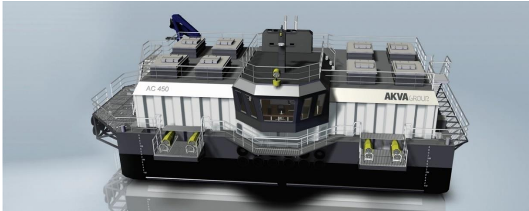
Figure 13 Feed Barge for salmon farms (AC 450), wind turbines and PV panels can be placed directly onto it, or floating by the side (AKVAgrouP, 2016)
