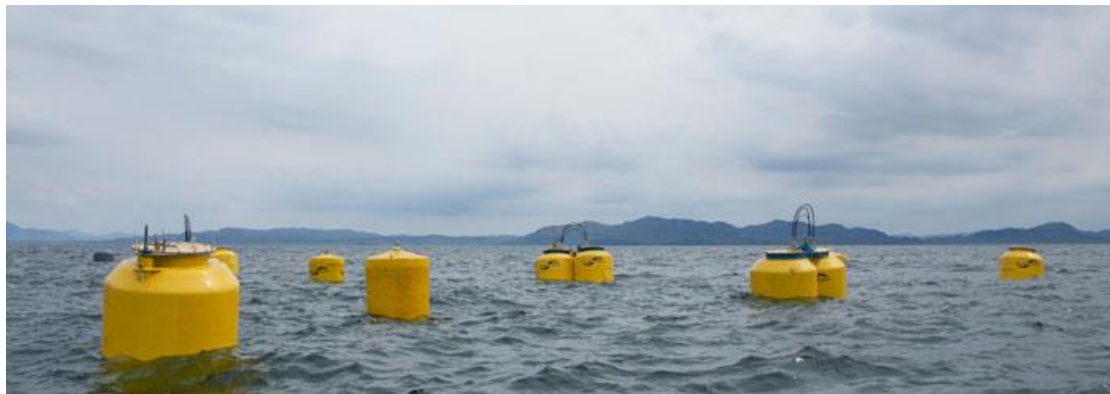
Figure 19 Albatern wave power project for a salmon farm in Scotland owned by Marine Harvest. A 22 kW wave energy converter device (WEC) was tested for 14 weeks in 2014 (Albatern Wave Energy, 2014).
