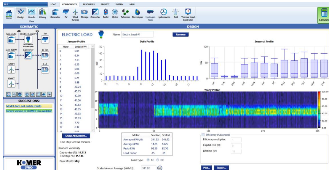
Figure 23 A screenshot of the HOMER energy interface. Here showing the system schematic in the top left corner, and the demand profile in the centre. Components can be added, demand profiles adjusted and results can be calculated.
