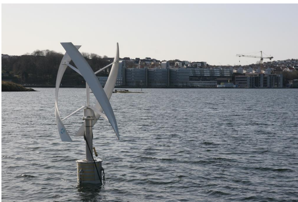
Figure 14 A floating 1 kW vertical axis wind turbine (VAWT), tested by Gwind outside Stavanger. VAWTs have a lower centre of mass, which could be beneficial for floating wind turbines (Gwind, 2014).
