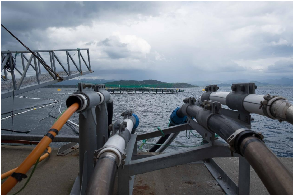
Figure 29 The hoses transporting the feed pellets out to the sea cages. The feed pellets are blown through the hoses using compressed air, before being spread out inside the sea cages.
