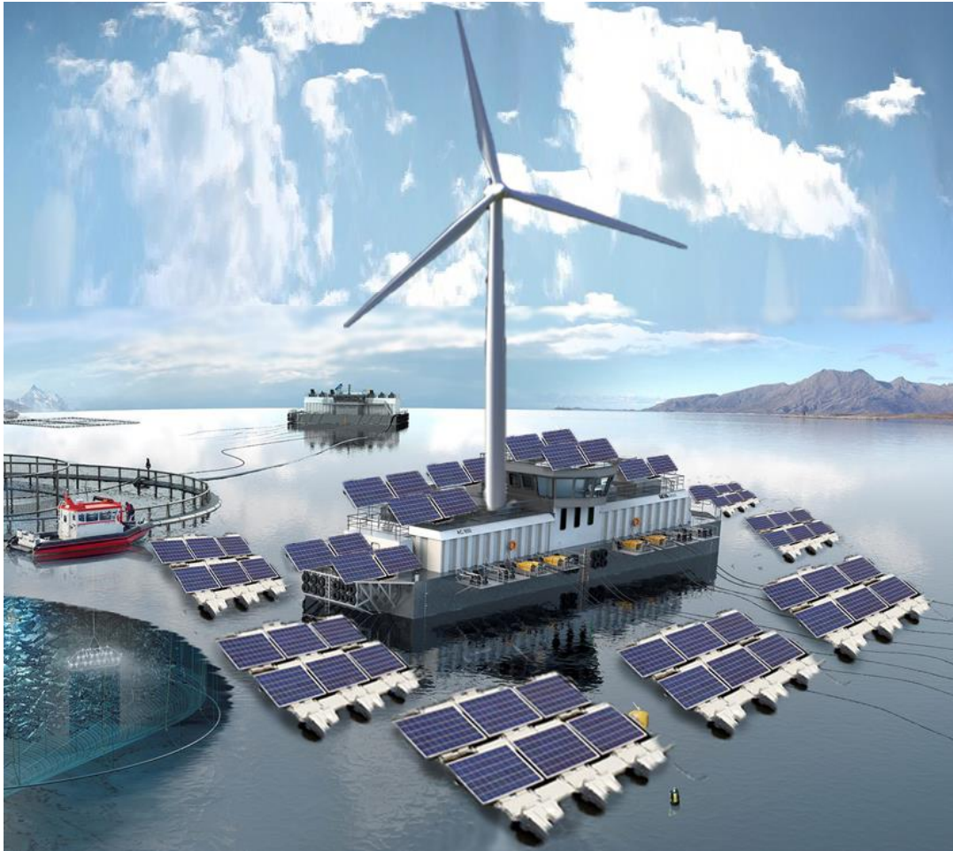
Figure 42 The feed barge with the 100% renewable system. The wind turbine has a capacity of 59 kW, and there is a total of 109 kW of PV capacity. Below deck there are Li-Ion batteries with a total capacity of 1,183 kWh and diesel generators. A lot of the PV panels are placed on floating modules as there is not enough space on the feed barge.
