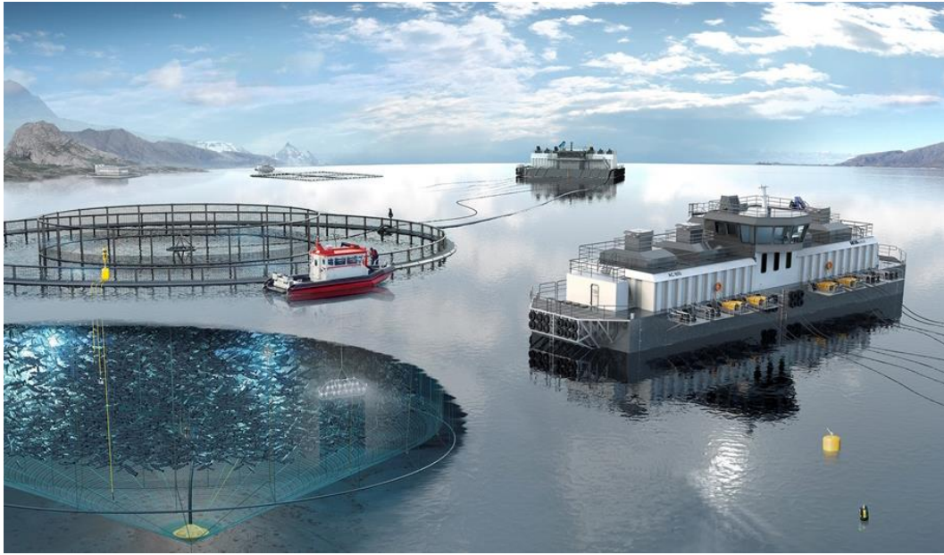
Figure 37 Illustration showing how a salmon farm can look today with a diesel generator. To the left is the net cage where the salmons are kept. To the right is the feed barge. The diesel generator and fuel is located below deck (Akva Group, 2015).
