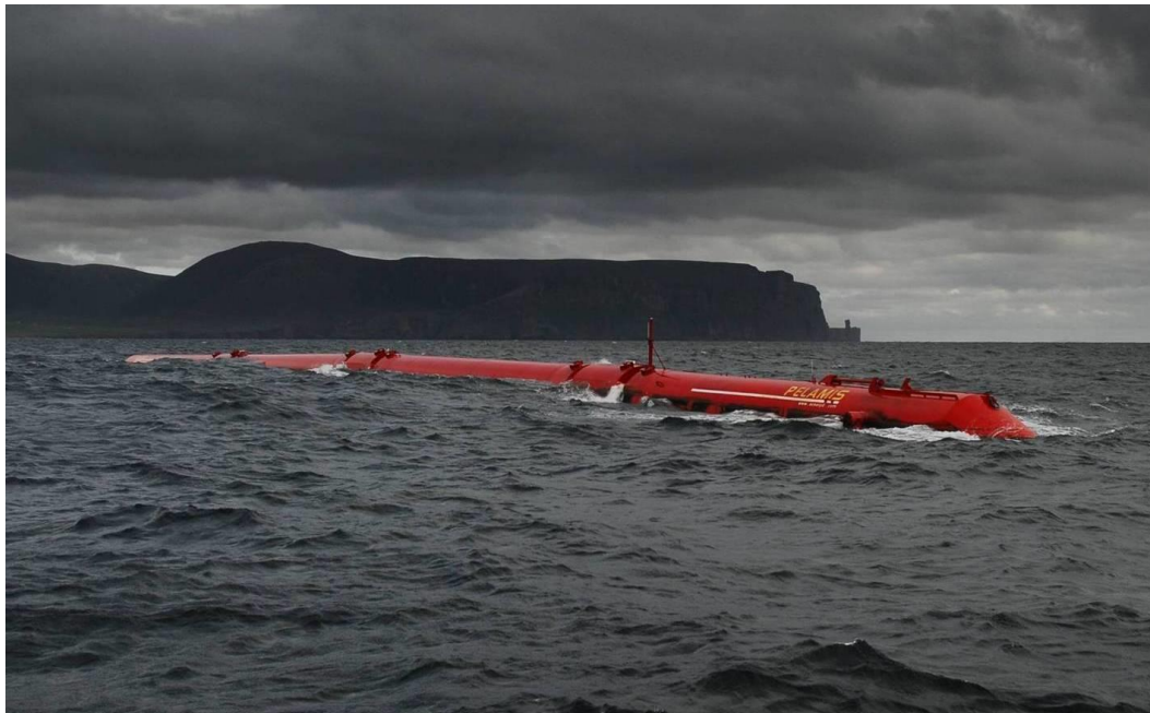
Figure 18 The 750 kW Pelamis P1 wave energy converter, located outside the Orkney Islands (Wikimedia public domain, 2014).
