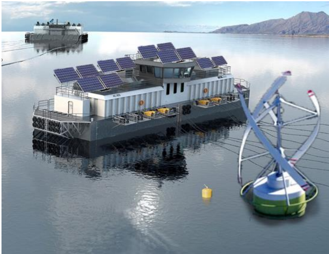
Figure 45 The feed barge with a floating vertical axis wind turbine (VAWT). Because of the different power curves for VAWTs and HAWTs, the systems with a HAWT were found to have a lower cost of electricity. However, VAWTs have a lower centre of mass, and as described in section 3.2.2, this could have benefits if the turbine is floating.
