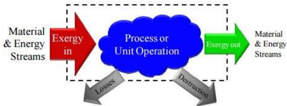
Figure 3. Exergy flows entering and exiting a Process or Unit Operation (Gundersen, 2011).
