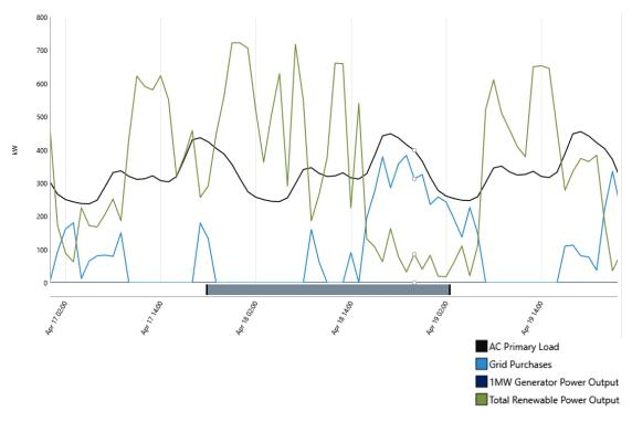
Fig 12. Power against time of wind-diesel-grid system
