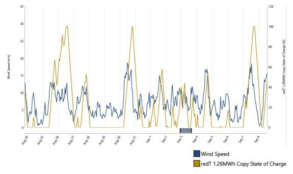
Fig 19. Effect of wind speed on battery's state of charge
