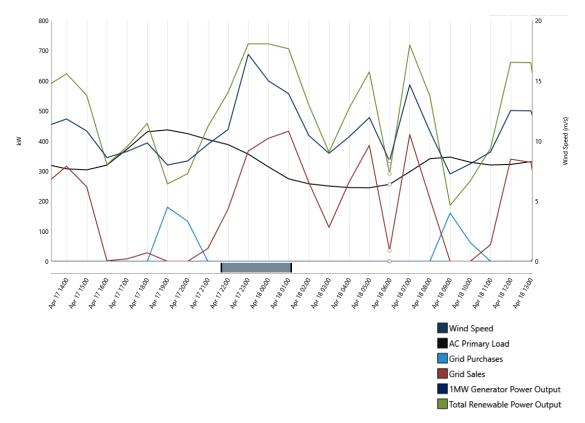
Fig 13. Graph showing rise in grid sales due to rise in wind speed
