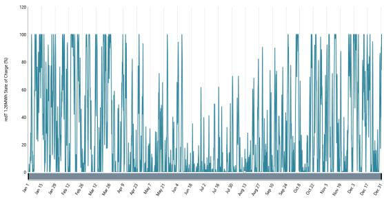
Fig 23. 420kW, 5040kWh battery's state of charge over a year
