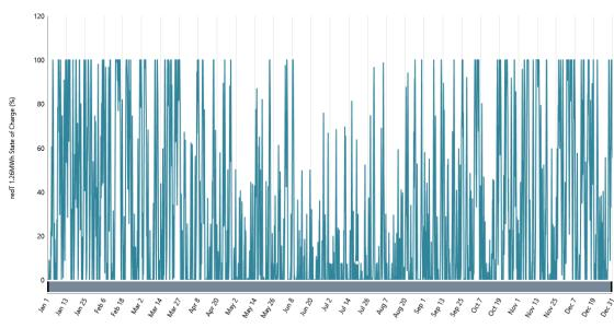
Fig 22. 105kW, 1260kWh battery's state of charge over a year
