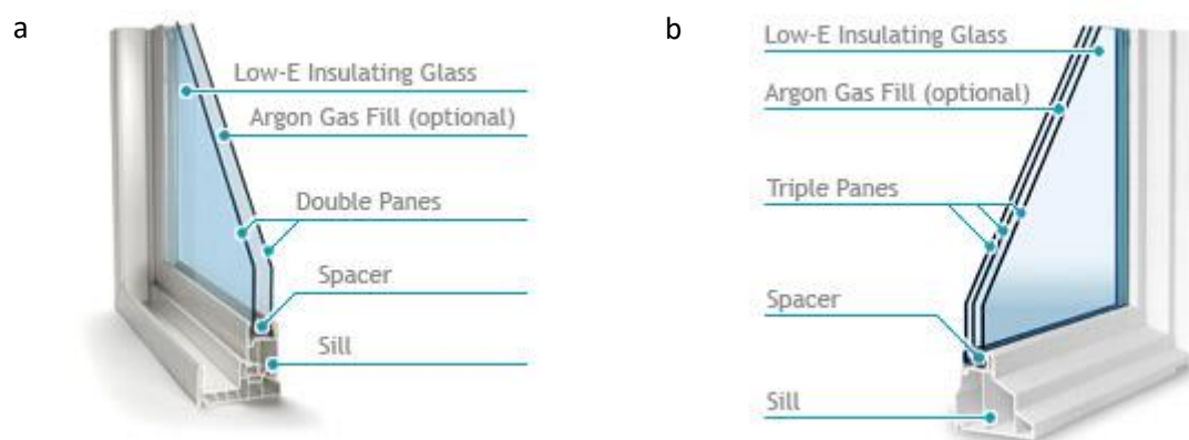
Figure 11: Depictions of a) double glazing and b) triple glazing windows (Milgard, 2016).
