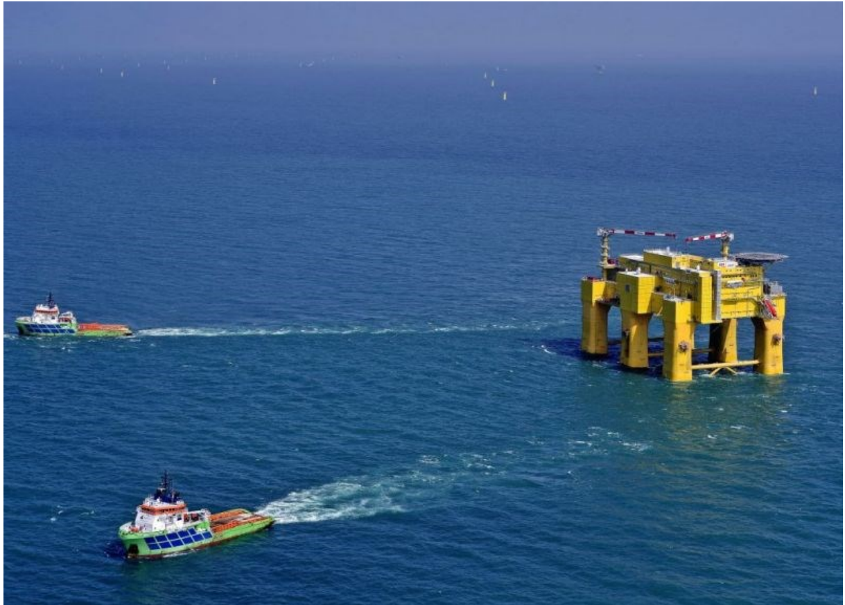
Figure 25: Dolwin Beta OSS transported by Semisubmersible bar (above) and transported by AHV (below) (29)
