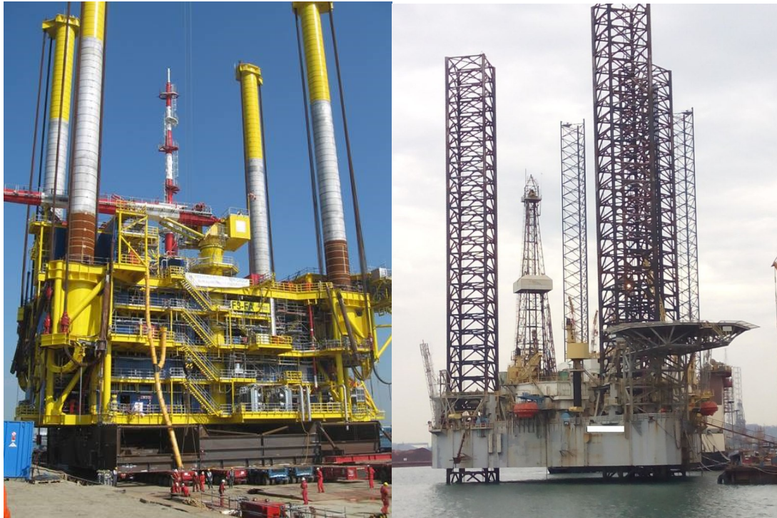
Figure 18: SEU with shell legs (left) (19). SEU with truss legs (right) (22)
