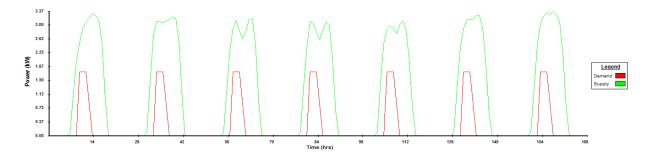
Figure 13: The Graph for small case model simulation in summer (35 unit of PV 100 W).
