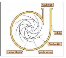
Figure 14 Francis Turbine Schematic Source: http://www.jfccivilengineer.com/
