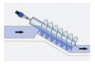
Figure 16: Reverse Archimedes Screw Source: http://www.energysavingadvisor.co.uk/
