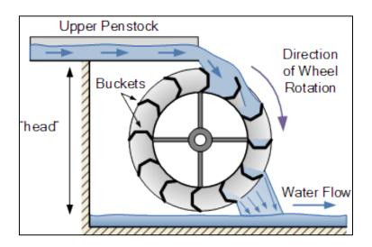
Figure 15: Overshot Waterwheel Operation
