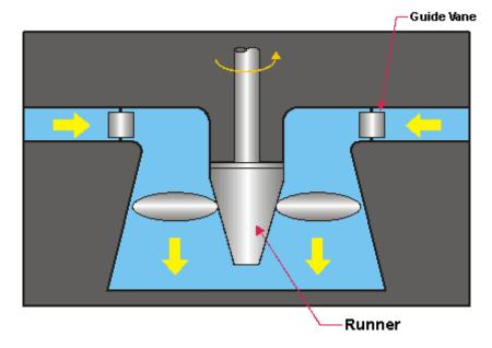
Figure 12: Propeller Turbine
