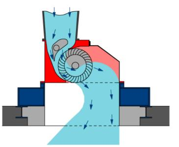
Figure 11: Crossflow Turbine
