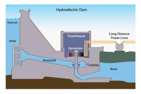
Figure 6: Operation of a hydroelectric dam
