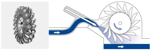
Figure 9: Pelton turbine and its operation
