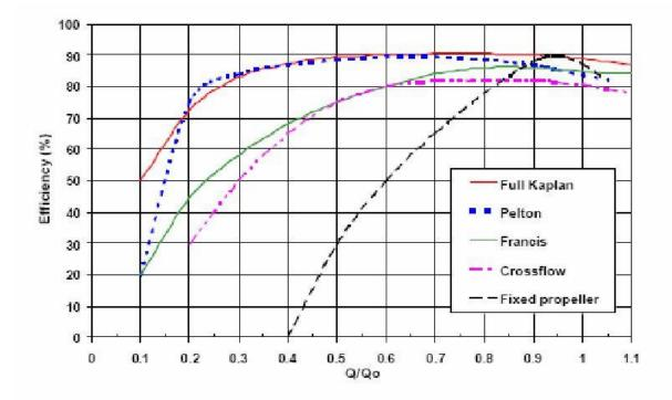
Figure 17 shows how the efficiency of selected turbines varies with the percentage of turbine flow.
