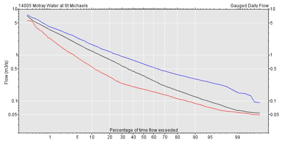
Figure 20: Flow Duration Curve for the Motray Water (2014)
