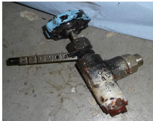
Figure 5 Galvanic Corrosion - Example 2
