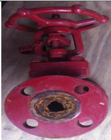
Figure 28 Cooling Water Isolating Valve
