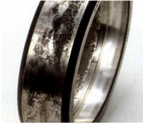
Figure 17 Fretting Corrosion Example 1 Figure 18 Fretting Corrosion Example 2
