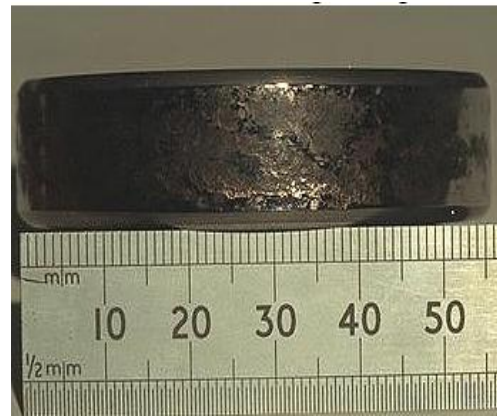
Figure 17 Fretting Corrosion Example 1 Figure 18 Fretting Corrosion Example 2
