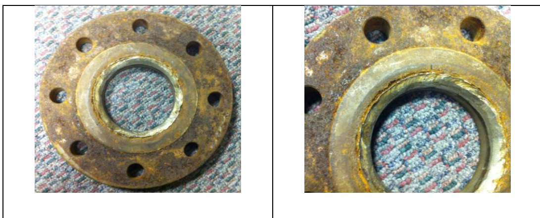
Figure 32 Flange from Power Station Visit – Galvanic Corrosion
