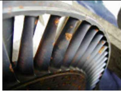
Figure 10 Pitting Corrosion Example 2
