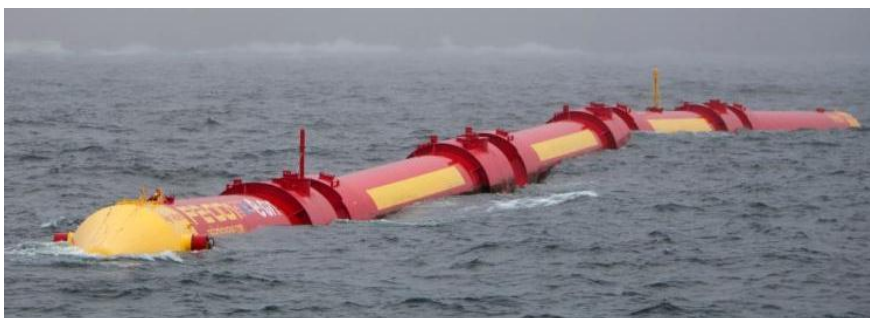
Figure 9 Pelamis P2 Being Tested in Open Water [49]
