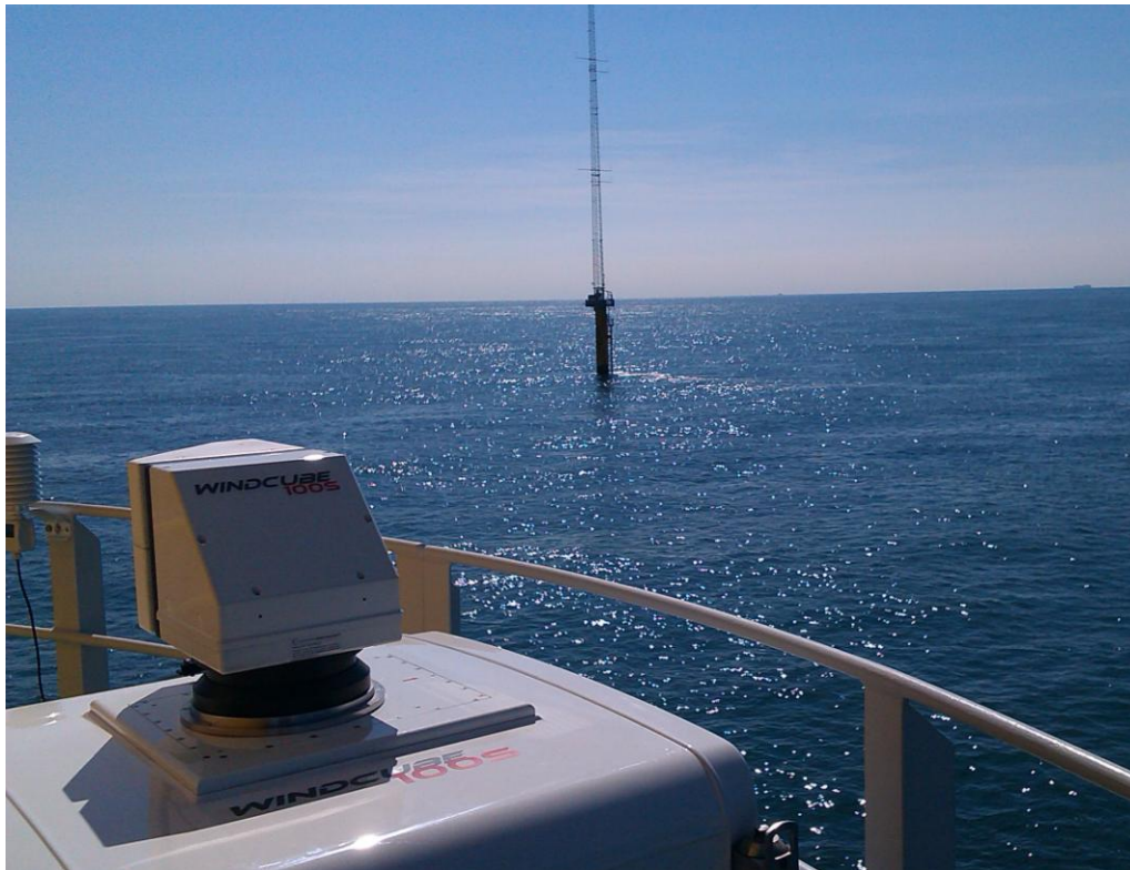
Figure 22: Location of LIDAR on Offshore Wind Turbine Transition Piece
