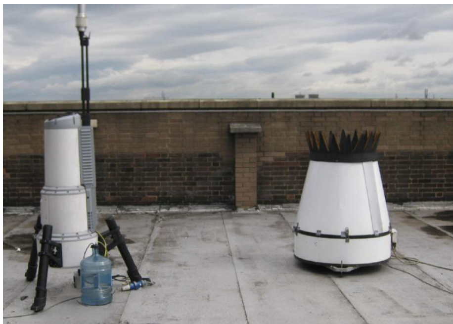
Figure 8: LIDAR and SODAR Example [13]
