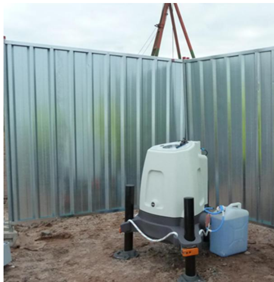
Figure 14: Onsite LIDAR Arrangement
