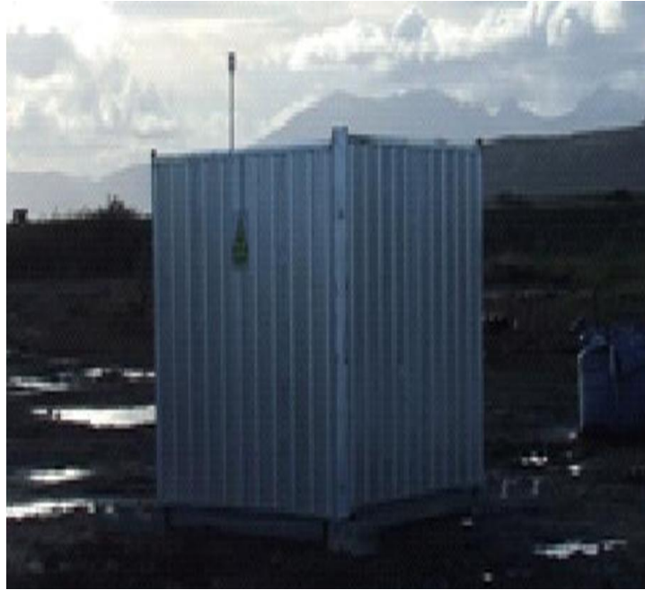
Figure 15: Onsite Security Fence Protection for LIDAR
