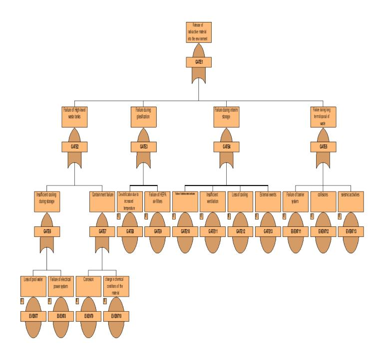
**Figure 5 : Fault tree showing different pathways leading to radioactive release**
