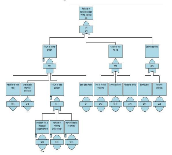
Figure 7: Fault tree model for failure during long-term disposal
