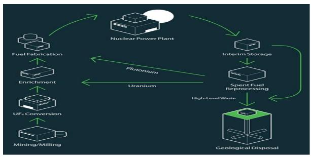
Figure 1: The Stages of a nuclear fuel cycle
