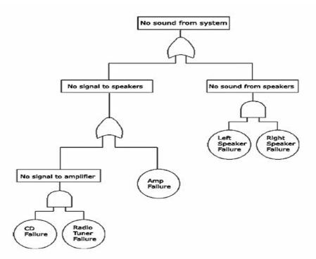
**Figure 4 : A simple fault tree**
