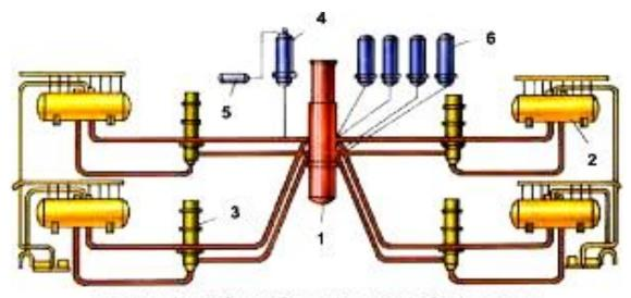
Reactor, 2. Steam Generator, 3. Main Coolant Pump,
