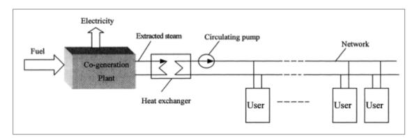
**Figure 1:1 – Basic Principle of District Heating (Lin et al., 2001)**
