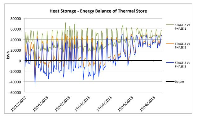
Figure 5:18 - Energy Balance of Heat Storage Vessel: Network Stage 2
