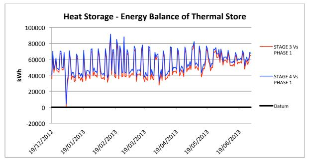
Figure 5:21 - Energy Balance of Heat Storage Vessel: Phase 1 v Stages 3&4
