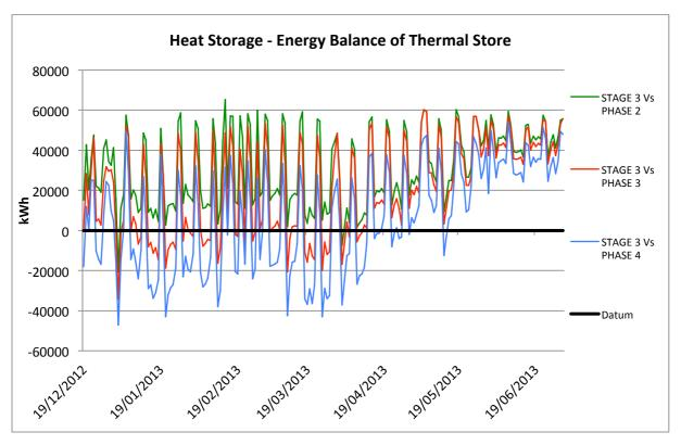
Figure 5:19 - Energy Balance of Heat Storage Vessel: Network Stage 3
