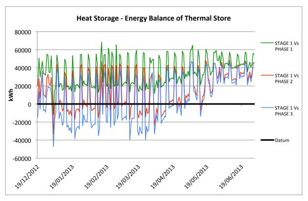
Figure 5:17 - Energy Balance of Heat Storage Vessel: Network Stage 1
