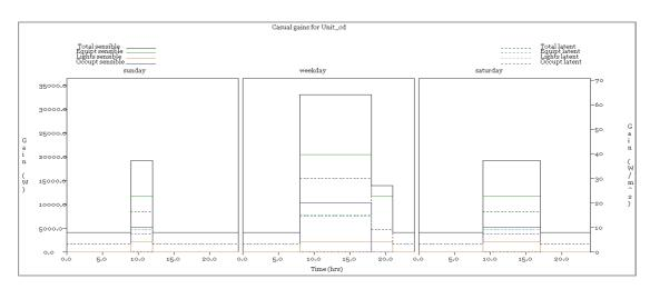
Figure 4:7 - Illustration of Esp-r Internal Gains Profile
