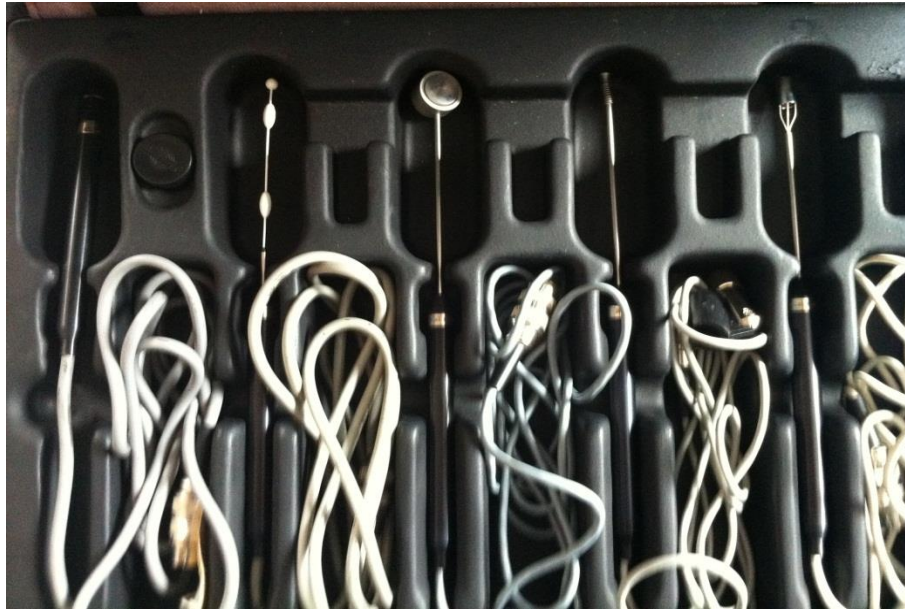
Figure 3.2 – The five transducers used for the indoor climate analysis. From Left to right: air temperature, surface temperature, air velocity, humidity, radiation
