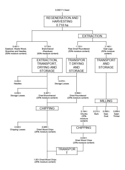
Figure 3: Biomass/process flow diagram for small-scale production of wood chips from woodland management (5)
