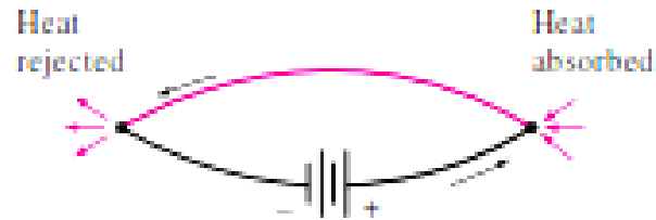
Figure 31: Peltier Effect, Source (Cengel & Boles, 2006, p.636)
