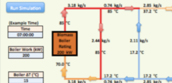
Diagram: Flow rates and temperatures through the biomass boiler system
