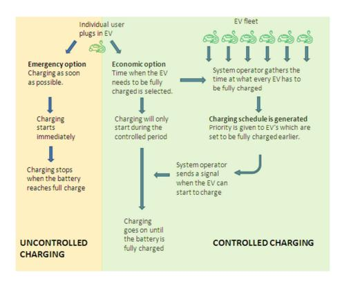
Figure 17: High level flow of the charging algorithm (own elaboration)
