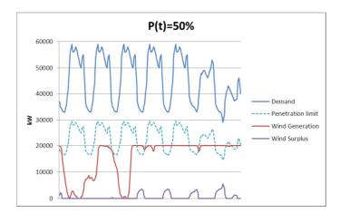
Figure 11: Example graph of the wind surplus calculation taking into account the wind power penetration limit, in this case 50% (own elaboration)
