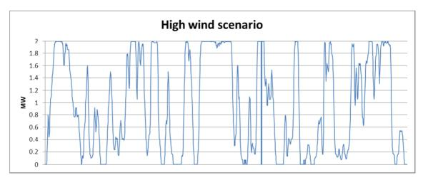
Figure 24: Wind power generation of a V80-2MW turbine during a month in the three posible scenarios analysed. (own elaboration)
