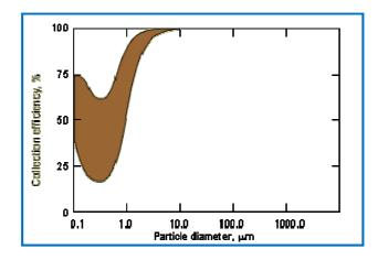
Figure 6: Particle size-Efficiency of wet scrubbers. SOURCE: US EPA [Ref.59].
