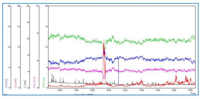
Figure 17: Concentration of air pollutants versus time at minimum heat output. *SOURCE:* [*Ref. 32*]
