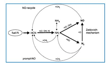
Figure 11: Reaction path diagram for NOx formation and destruction in the gas phase. *SOURCE:* [*Ref.53*]
