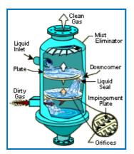
Plate scrubber: Working with the same mechanism, in this system the gas atomises the entering water by the acceleration caused by tiny holes in the horizontal plates. The gas-water contact is counterflow, as the water is scrubbed in the top and the gas flows from the base. Figure 4 shows a plate scrubber system:
