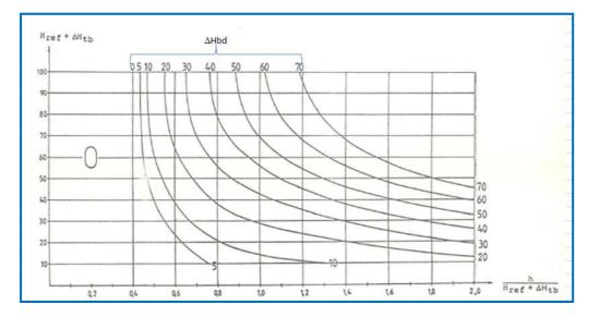
Figure 25: Diagram to calculate  $\Delta$ Hbd
