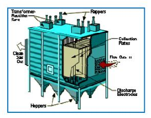
Figure 7: Electrostatic precipitator. SOURCE: US EPA [Ref.59].
