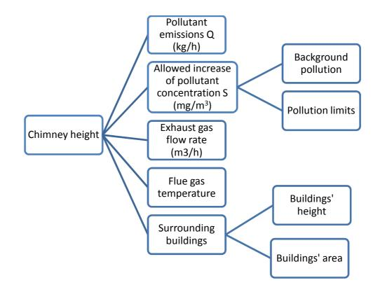
Figure 38: Diagram showing the relationship of the parameters influencing chimney height for the Austrian calculation procedure.
