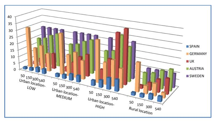
Figure 42: Chimney heights obtained by the different European methodologies.
