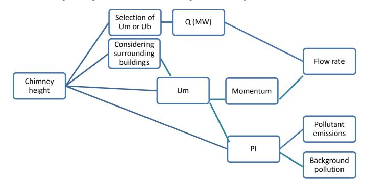
Figure 32: Diagram showing the relationship of the parameters influencing chimney height for the UK calculation procedure.
