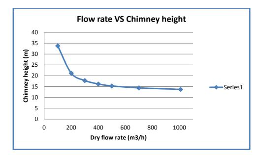
Figure 40: Relationship between the flow rate and the chimney height, according to the results obtained following the German method.
