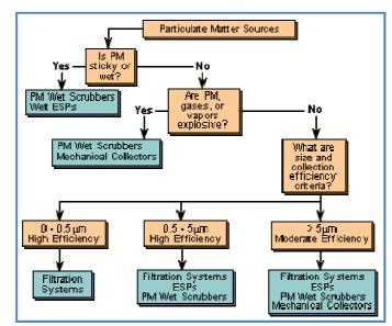
Figure 10: Guidance for PM removal system selection. SOURCE: US EPA [Ref.59].
