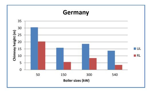
Figure 39: Chimney height calculation results for the created case studies following the German methodology.
