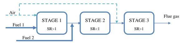
Figure 13: Three- stage combustion process.
