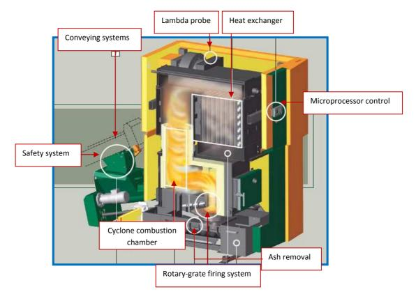
Figure 15:KWB TDS POWERFIRE 150 boiler. SOURCE: Boiler test report [Ref.33].
