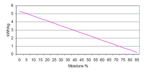
The high moisture content will decrease the lower heating value of the biomass fuel and in turn affect the fuel efficiency, as well as the size of the boiler. Therefore a more expensive boiler has to be installed, if the moisture content is high.
