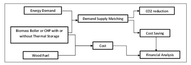
This figure illustrates the main methodology this tool considers in order to assess the feasibility of using waste wood as biomass fuel for the boiler and CHP.
