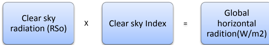
Figure 25: Global horizontal radiation calculation procedure
