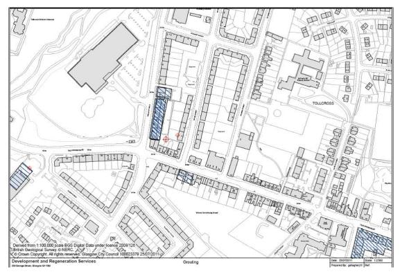
Fig 6.1.6. Grouting plan for Wellshot road. (supplied by Glasgow City Council) The dashed blue rectangle along Wellshot Road is the grouted area and the red crosshair is the location of the Mutton Pit.
