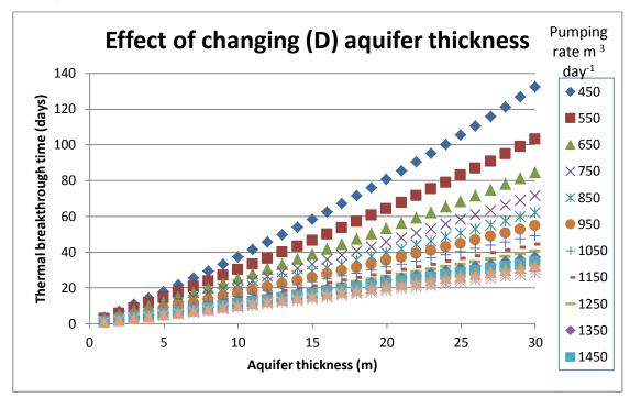
Fig 6.5.9 Thermal breakthrough time in relation to pumping rate and aquifer thickness.
