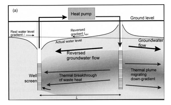
Fig 4.2. Well doublet experiencing thermal feedback (Banks 2008, p170)
