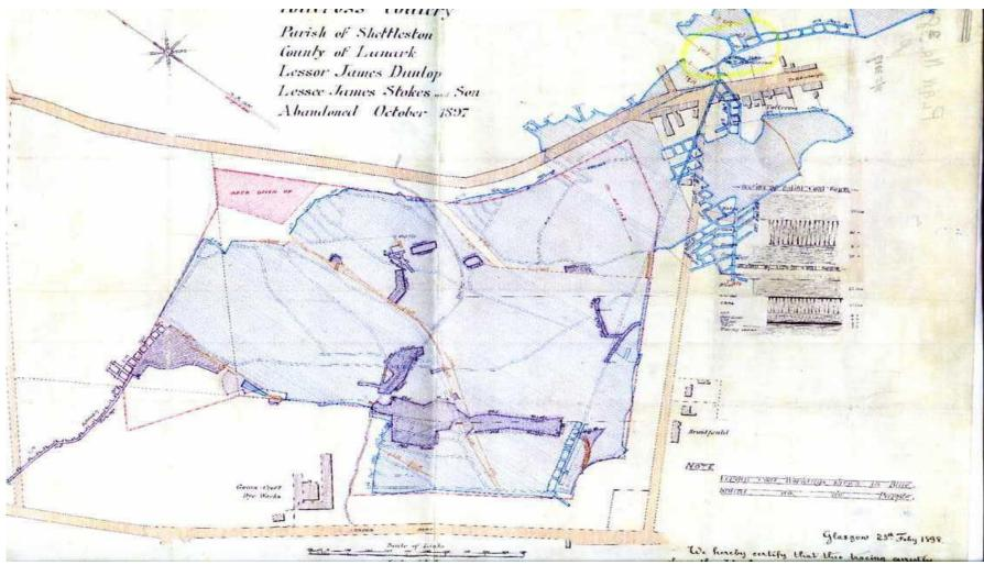
Fig 6.1.5, Large abandonment plan showing the connection between the Mutton pit and the rest of the worked Virgin seam in this area (Supplied by the BGS)
