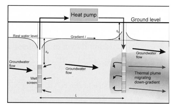
Fig 4.1. Well doublet with no thermal feedback (Banks 2008, p167)
