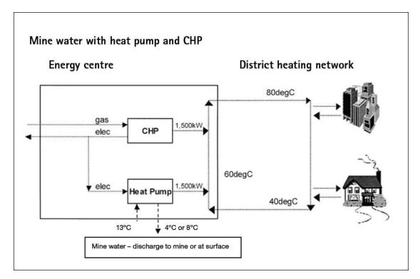
Fig 2.5.1. Heat pump and CHP heating system (taken from minewater project paper)
