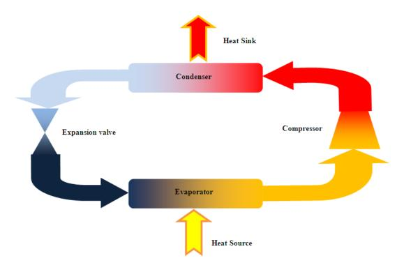
Fig 2.2.1. Components of a heat pump
