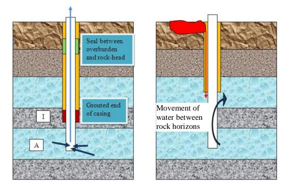
Fig 3.3.1, Two scenarios showing the potential hazards involved in the casing of a borehole.
