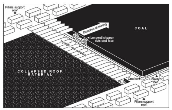
Fig 2.3.2. Longwall mining (taken from <u>http://rajikorba.blogspot.com/2011/06/long-</u>wall-technology-in-coal-mines.html)
