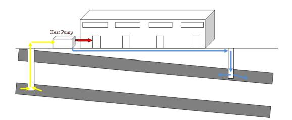
Fig 2.2.2 Open source system for a block of flats
