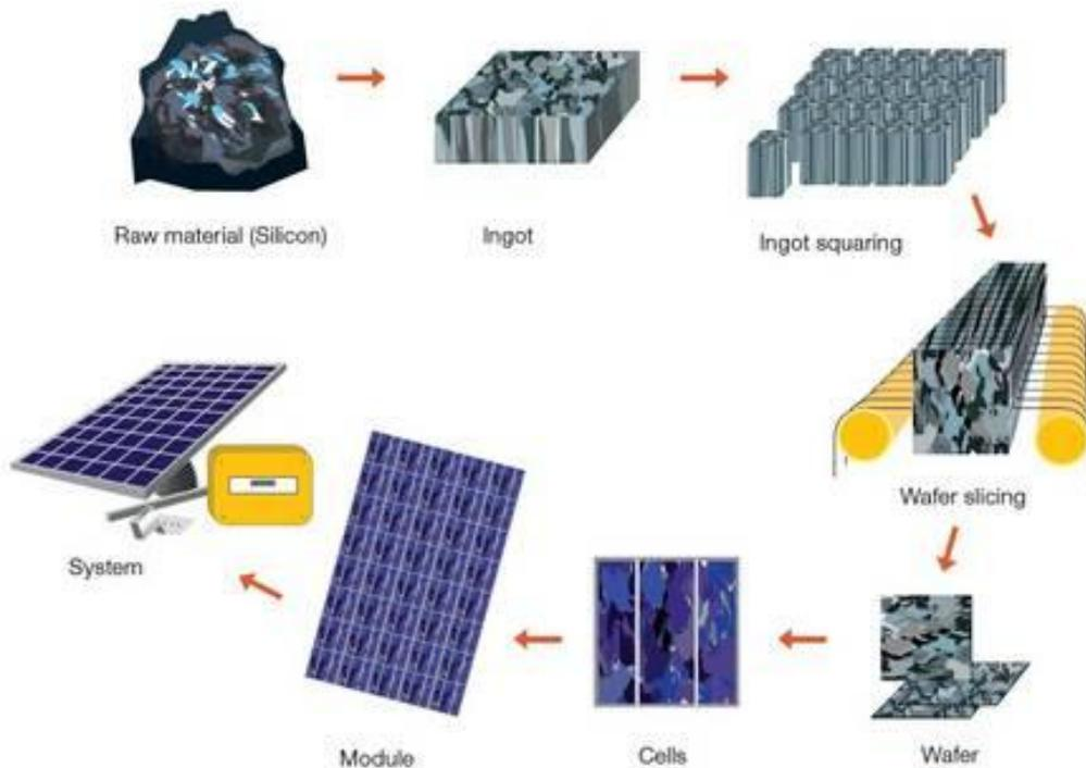
**Figure 12:** PV production procedure
