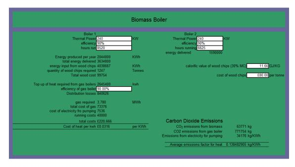
Figure 29 Carbon calculator – biomass boiler
