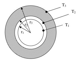
Figure 11 Composite cylinder
