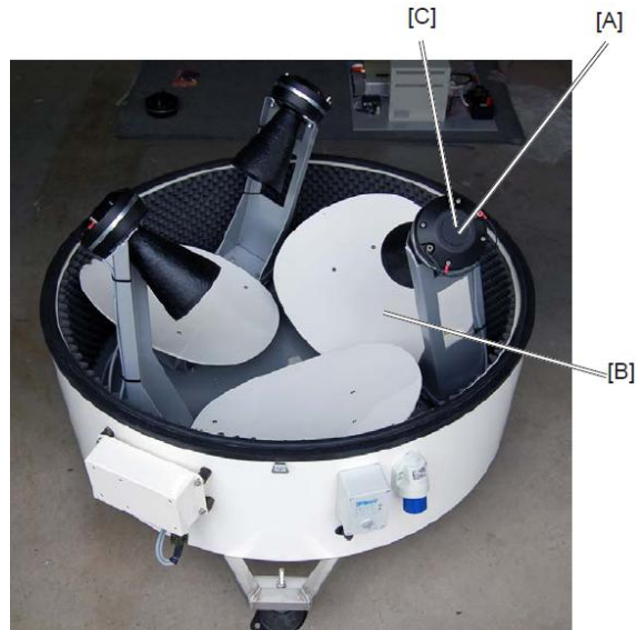
Figure 20: Internal view of SODAR device
