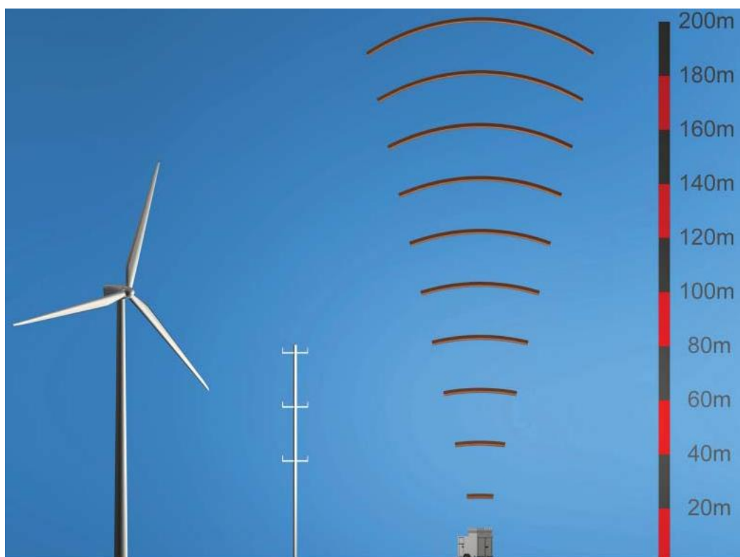
Figure 8: SODAR and Anemometer measuring wind
