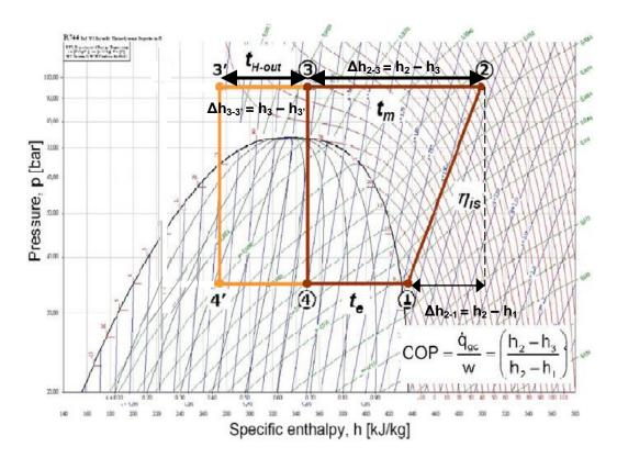
Figure 4.1.2.1.1 P-h diagram for COP of a transcritical CO<sub>2</sub> heat pump cycle with internal heat exchanger
