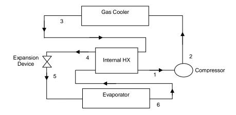
Figure 1.5.1 Layout of transcritical CO<sub>2</sub> system with internal heat exchanger
