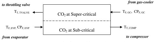
Figure 4.2.1.3.1 Principle of internal heat exchanger sub-section
