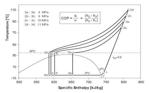
Figure 4.1.3.3.1 the transcritical CO<sub>2</sub> heat pump cycle operated at four different high-side pressures and gas-cooler outlet temperature assumed to be constant at 35°C (Source:CO<sub>2</sub> heat pump for combined SH and DHW)
