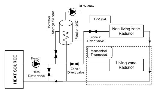
Figure 3.1.4.1 Schematic diagram of control system modelled in chosen house type (Source: Report on ADEPT by ESRU, 2007)
