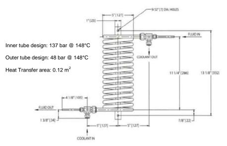
Figure 4.2.1.2.1 Sentry-equip made tube-in-tube counter flow gas-cooler (source: Sentry-equip, Model no. DTC-CUA/CUA-4-1-1)
