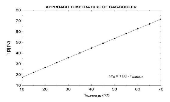
Figure 4.2.3.2.4 Graph showing the effect of hot water return temp. on refrigerant exit temperature in gas-cooler, their difference is denoted as  $\Delta T_A$ . developed using EES
