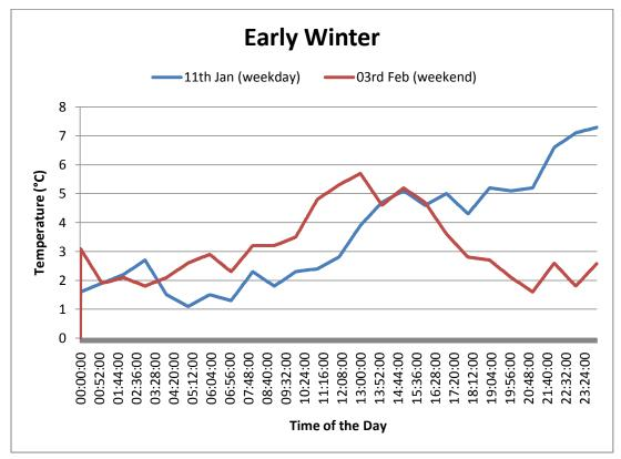
The following graphs show the atmospheric temperature of days in different seasons used for simulation of heat pump to investigate its seasonal performance factor.
