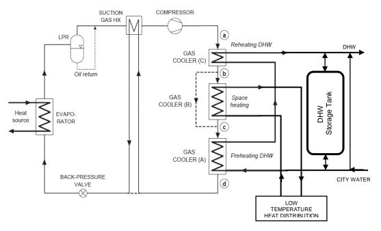
Figure 2.2.1 Principle design of Integrated CO<sub>2</sub> heat pump for space and DHW heating for Passive housing
