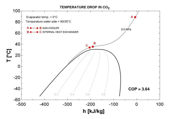
Figure 4.2.3.2.3 Temperature glide in gas-cooler, for water side temperature of 80/30°C at a high-side pressure of 8.5 MPa. Developed using EES
