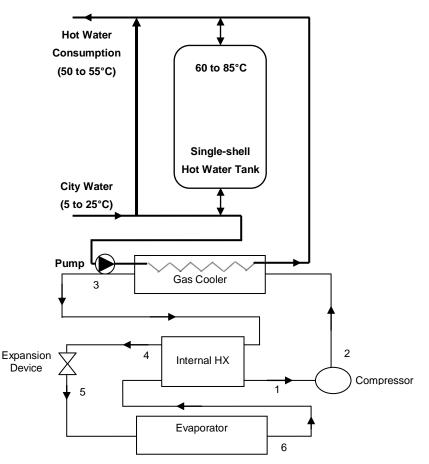
Figure 2.1.1 Simple CO<sub>2</sub> heat pump water heater
