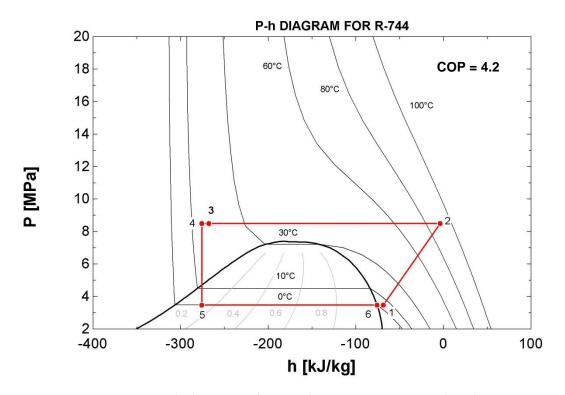
Figure 4.2.3.2.6 P-h diagram of a  $CO_2$  heat pump system, when hot water temperature profile 80/10°C, high-side pressure of 8.5 MPa. Developed with EES
