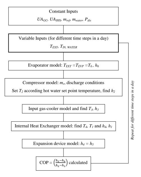
Figure 4.2.2.1.1 Flow chart for the numerical simulation
