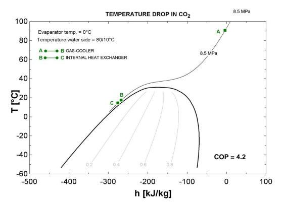
Figure 4.2.3.2.2 Temperature glide in gas-cooler, for water side temperature of 80/10°C at a high-side pressure of 8.5 MPa. Developed using EES
