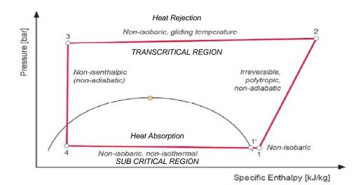
Figure 1.4.2 Transcritical CO<sub>2</sub> heat pump cycle (Lorentzen cycle) P-h diagram (Source: J.Stene, Intergrated CO<sub>2</sub> heat pump for space and hot water in passive houses)
