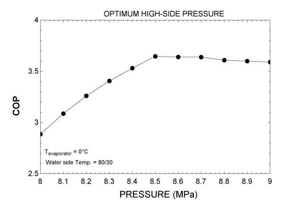
Figure 4.2.3.1.1 Graph for COP vs. PRESSURE to find Optimum high-side pressure of the transcritical CO<sub>2</sub> heat pump cycle, developed using EES
