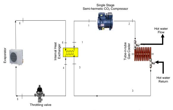
Figure 4.2.1.1 Transcritical CO<sub>2</sub> Heat pump simulator
