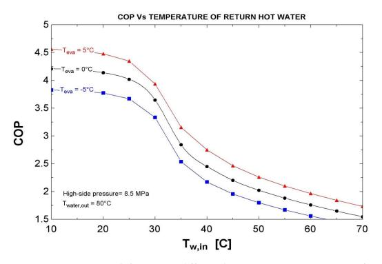
Figure 4.2.3.2.5 Graph for COP at different hot water return temperatures for different evaporator temperatures. Developed using EES.
