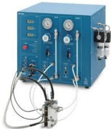
Figure 4.3.4 FCT-50S and FCT-150S Fuel Cell Test Station for PEMFC
