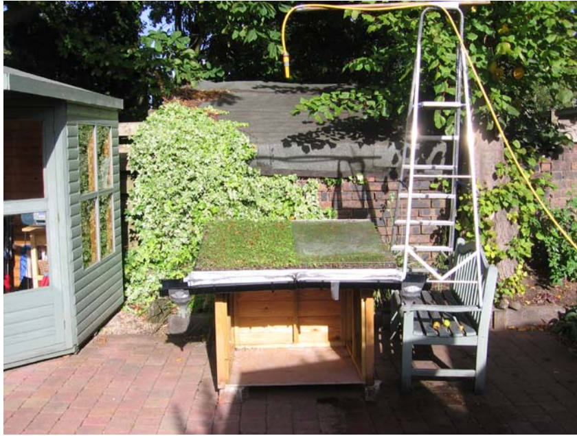
Figure 40: Green Roof Test Rig for Rainfall Runoff with Sprinkler
