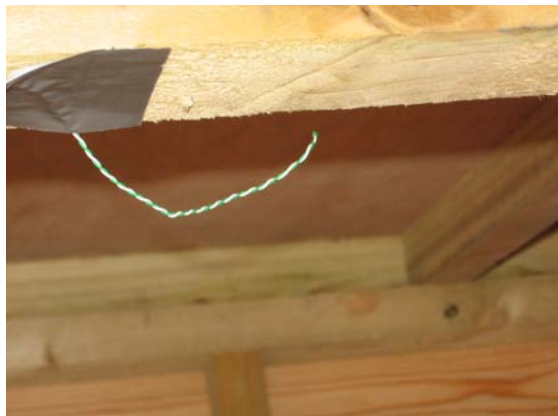
Figure 26: Under Roof and Substrate Thermocouple Placement
