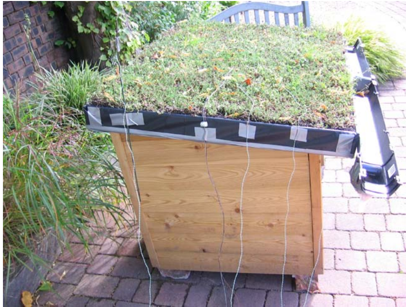
Figure 28: Green Roof Thermocouple Placement
