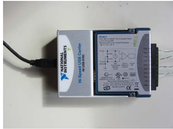
Figure 25: NI USB-9211 Thermocouple Attachment
