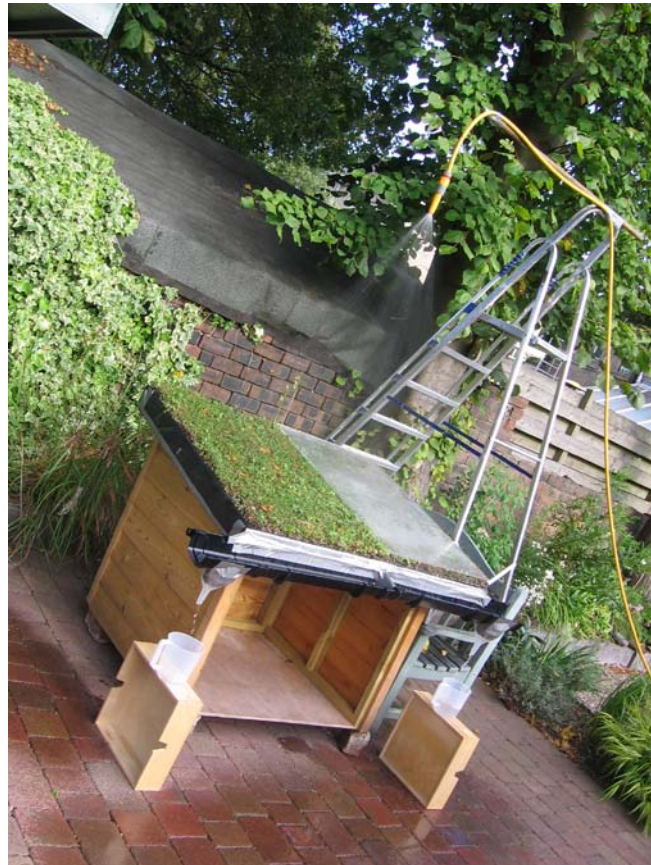
Figure 39: Green Roof Test Rig for Rainfall Runoff with Artificial Rain Event
