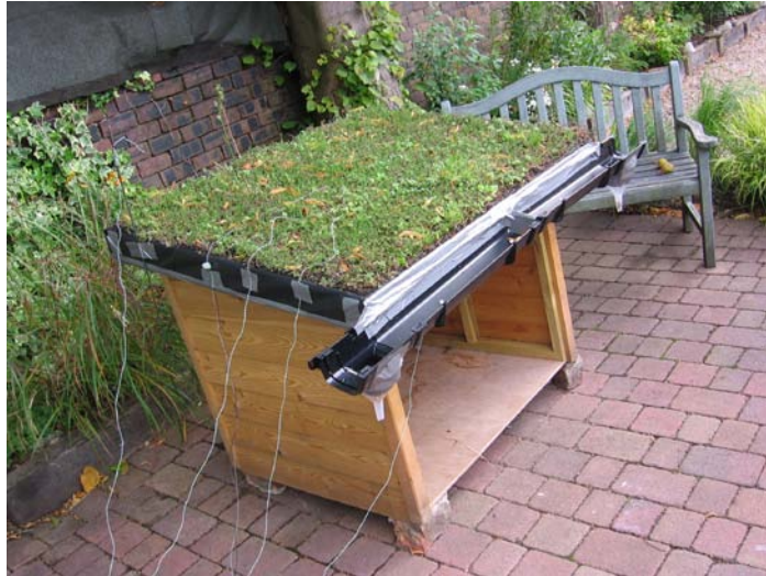
Figure 21: Green Roof Test Rig
