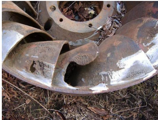
Fig. 4.16: Francis Turbine showing cavitation damage (Source: [40])
