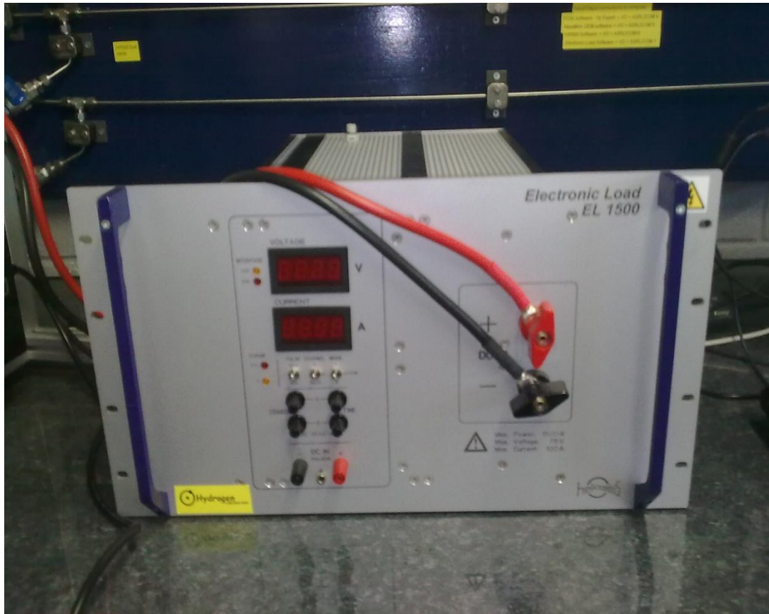
Figure 28 - Electronic Load on Fuel Cell
