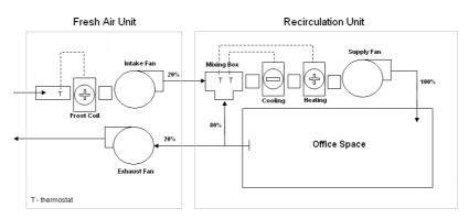
Figure 39: VAV and CAV system diagram
