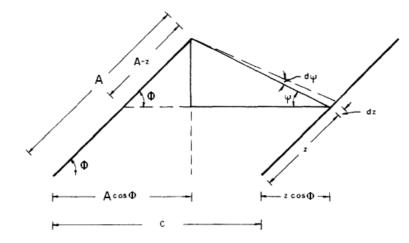
Figure 57: Diffuse beam shading impact from adjacent panels (from Passias et al. [72])
