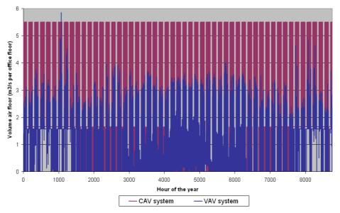
Figure 40: Volume flow rate for CAV and VAV systems
