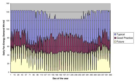
Figure 41: Fan energy requirement comparison between the different office scenarios
