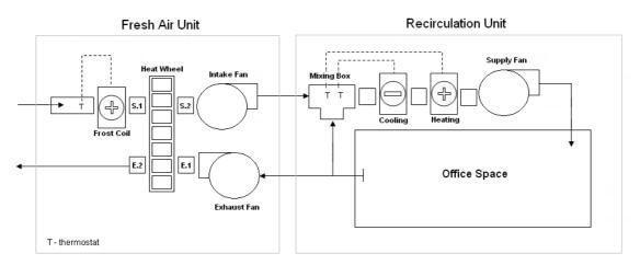
Figure 42: HVAC system with Heat recovery wheel in the Fresh Air Unit
