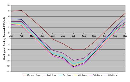
Figure 37: Monthly averaged heating and cooling loads of the building
