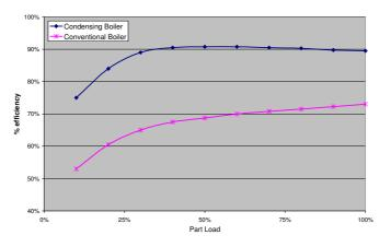
Figure 43: Boiler Part-load performance
