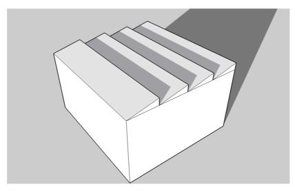
Figure 55: Shading occurring on rooftop PV panels
