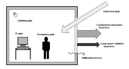
Figure 34: ESP-r heat flux balance in each zone
