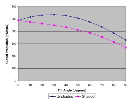
Figure 63: Global irradiation for panels at different tilt angles in London
