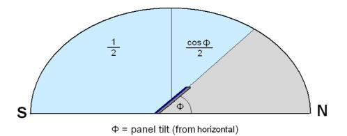
**Figure 54: North-south section explaining diffuse radiation on tilted panels** Diffuse radiation on a tilted panel on the roof:
