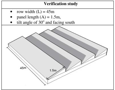
Figure 59: Roof PV layout
