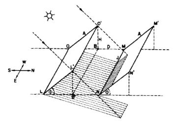
Figure 56: Direct beam shading from adjacent panels (from Appelbaum et al. [73]) The shaded direct beam ( $I_{BS}$ ) is then calculated from:
