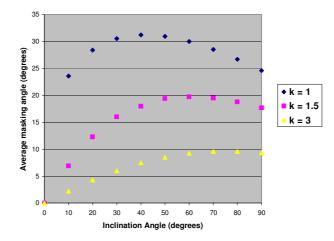
**Figure 58: Average masking angles vs. inclination angle for various values of C/A (=k)** Overall diffuse irradiance is recalculated taking into account this average masking angle:
