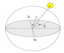
Figure 53: Explanation of solar azimuth and elevation [75]
