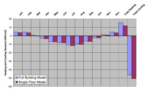
Figure 38: Verification of single floor model
