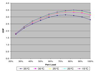
Figure 44: Conventional chiller system COP
