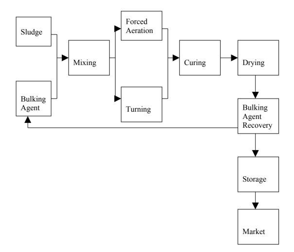
Figure 1: Composting Process Flow Diagram [1]
