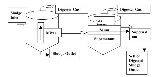
Figure 6: Two stage Digester [1]
