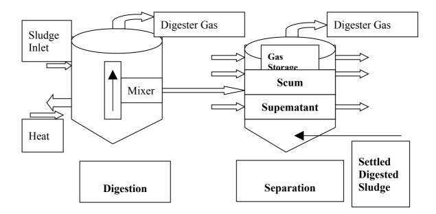
Figure 3: Complete mix, or high rate, anaerobic digester [17]
