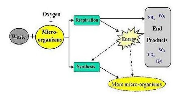
Figure 5: PATH of aerobic digestion [20]
