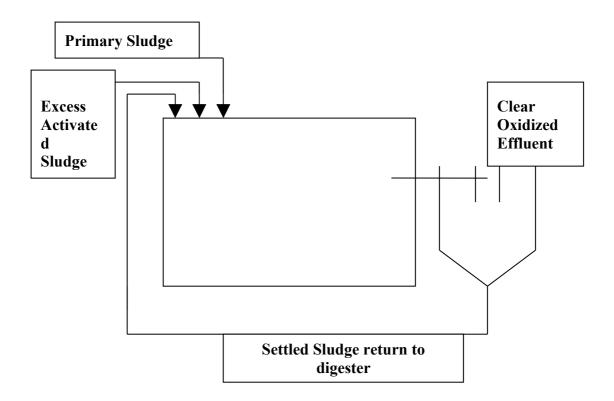
FIGURE 7: SCHEMATIC OF AEROBIC SLUDGE DIGESTION [1]
