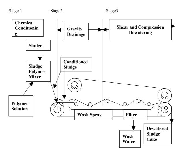
Figure 2: Belt Filter Press [1]
