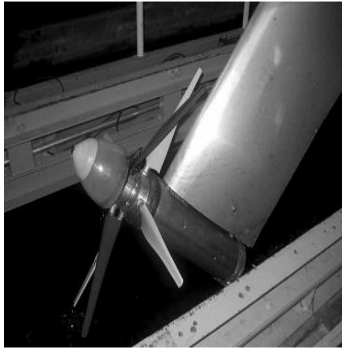
Figure 3: ESRU's CoRMaT design on test rig
