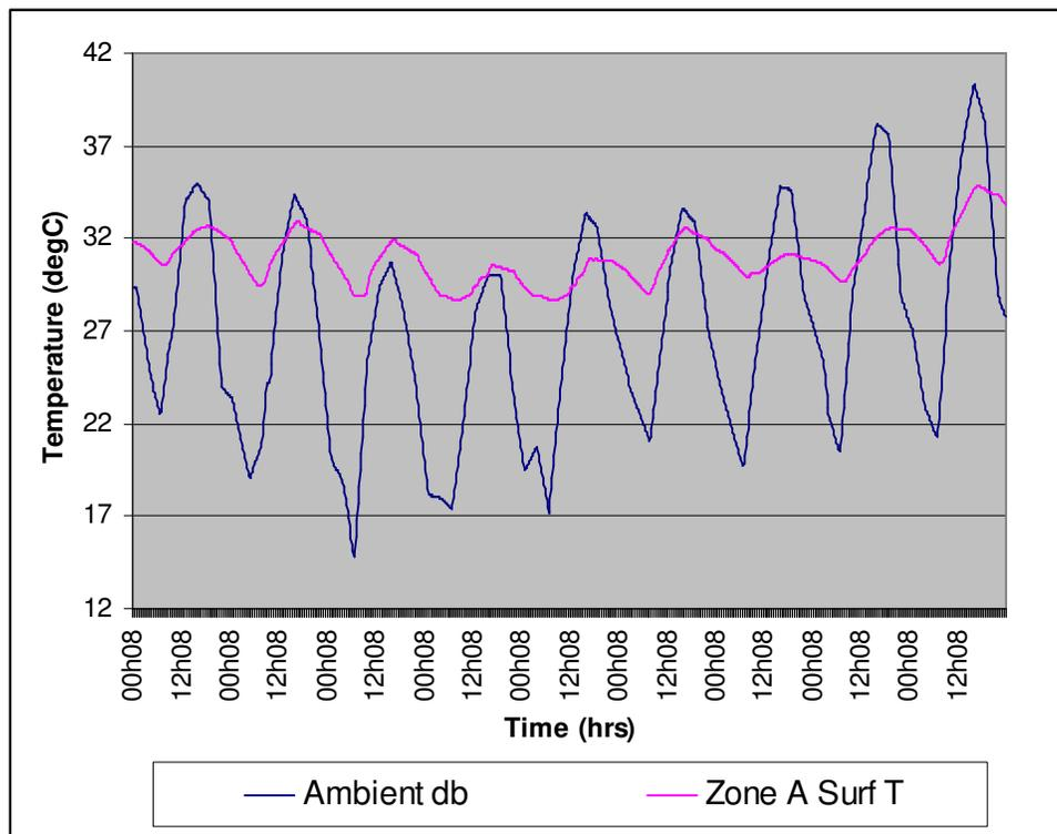
**Figure 17** Response of Wall-4 temperature to ambient db temperature. Period 12<sup>th</sup> - 20<sup>th</sup> August.
