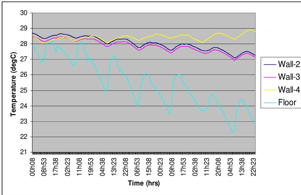
**Figure 20** Wall Surface Temperatures when PCM2 was applied.
