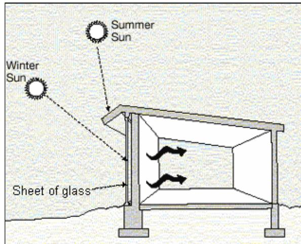
**Figure 3** Schematic of a Trombe Wall.<sup>3</sup>
