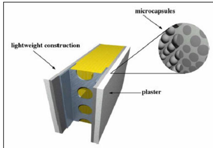
**Figure 4** Schematic of a lightweight PCM wallboard.<sup>4</sup>
