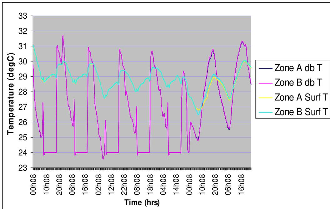
**Figure 14** Surface and Internal db Temperatures for Wall-3 with and without PCMI
