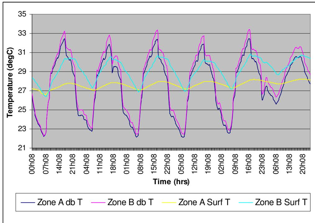
**Figure 16** Surface Temperatures of Wall-4 and Internal db Temperatures. Period 25<sup>th</sup>-30<sup>th</sup> June
