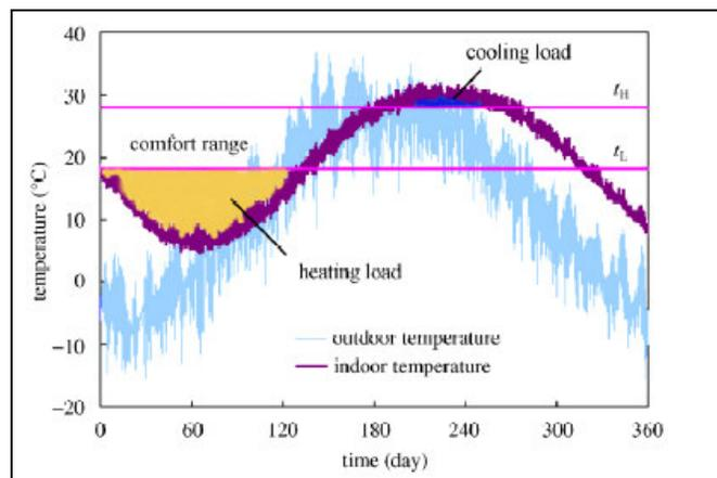
**Figure 1 Heating and Cooling load profile in a building environment;<sup>1</sup>**
