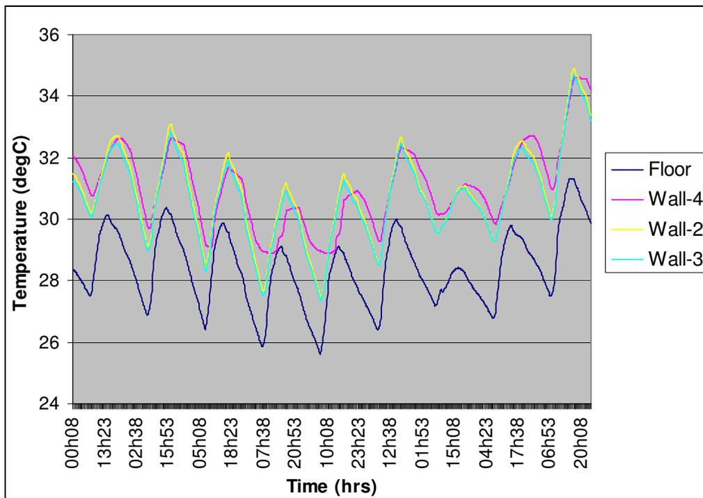
**Figure 18** Effect of PCM location on surface temperature.
