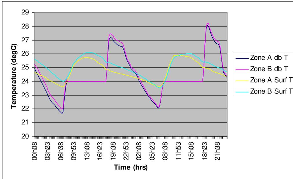
**Figure 24** Surface Temperature of Base-6 in both zones; Internal db Temperature. Period 23<sup>rd</sup>-24<sup>th</sup> August
