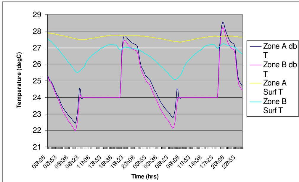
**Figure 22** Surface Temperature of Wall-3 in both zones; Internal db Temperature. Period 23<sup>rd</sup>-24<sup>th</sup> August
