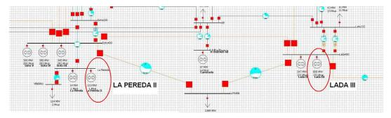
Figure 49. New Power World model generators (South)
