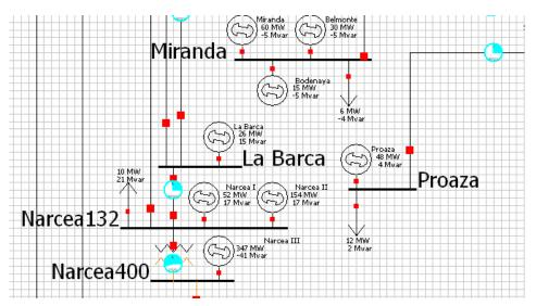
Figure 20. Power World model generators (South West)
