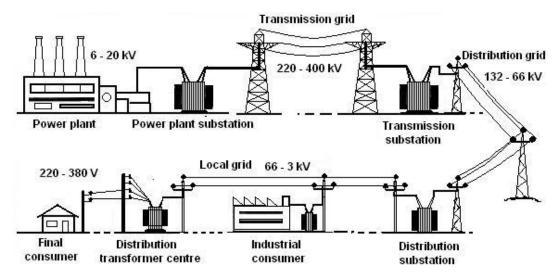
Figure 2. Electrical network structure [17]
