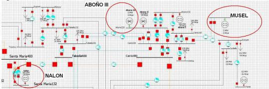
Figure 48. New Power World model generators (North)
