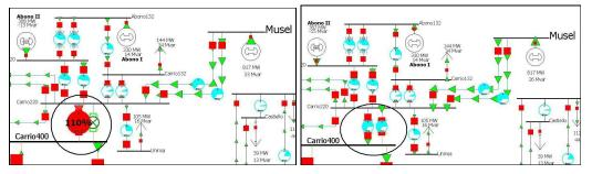
Figure 52. Simulations results after and before adding a second transformer
