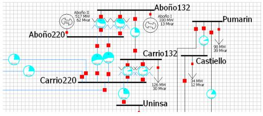
Figure 16. Power world model generators (North -Gijon)
