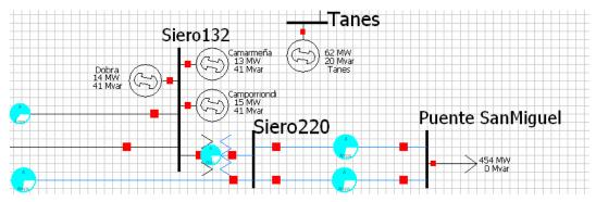
Figure 18. Power World model generators (East)
