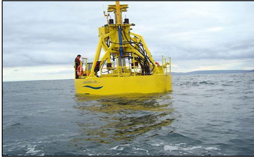
Figure 20 Point absorber devices (source: www.foxnews.com )
