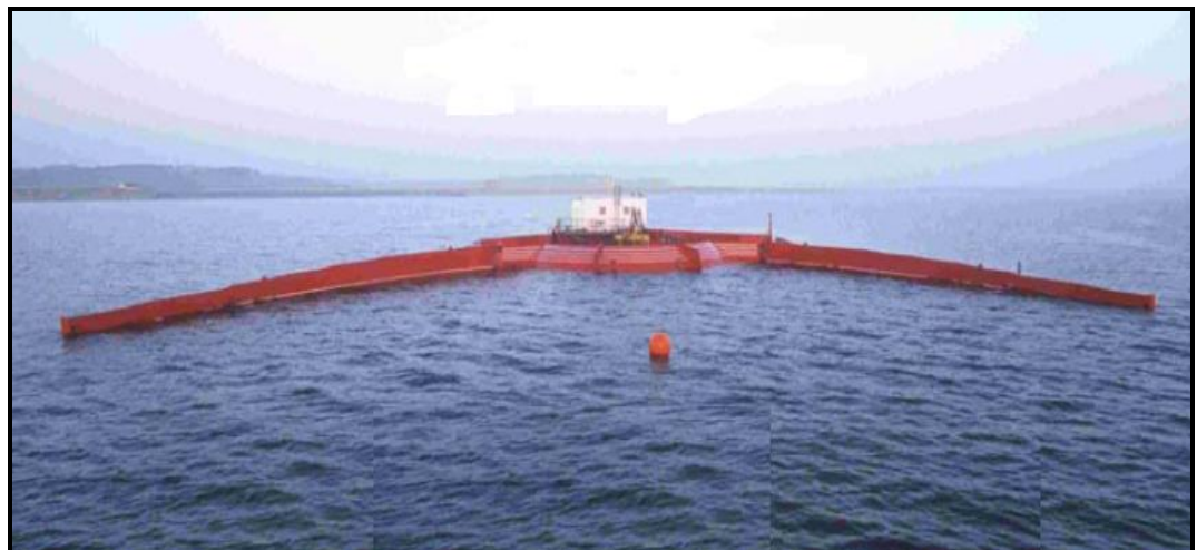
Figure 21 Overtopping devices (source: www.sut.org.uk )
