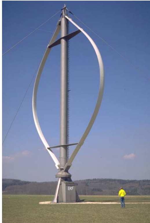
Figure 19: A Darrieus-type vertical axis turbine
