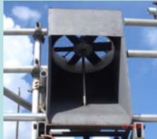
DWT mounted on the roof of James Weir Building and its power curve
