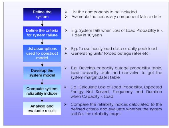
Figure 2-2: Reliability models construction process
