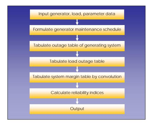
Figure 4-1: Flowchart for generating system reliability calculation (Source: Wang & McDonald, 1994)
