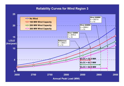
Figure 5-3: Wind Region 3 capacity credit evaluation using reliability curves
