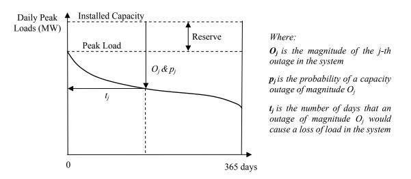
Figure 2-4: LOLP Calculation using Load Duration Curve
