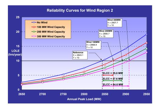
Figure 5-2: Wind Region 2 capacity credit evaluation using reliability curves
