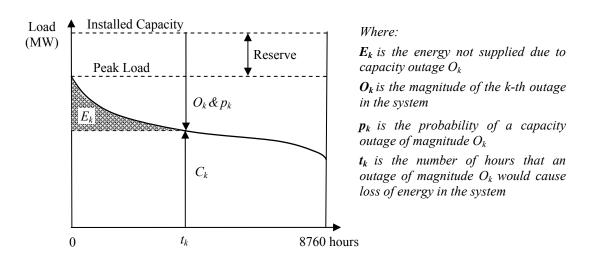
Figure 2-5: LOEP Calculation using Load Duration Curve
