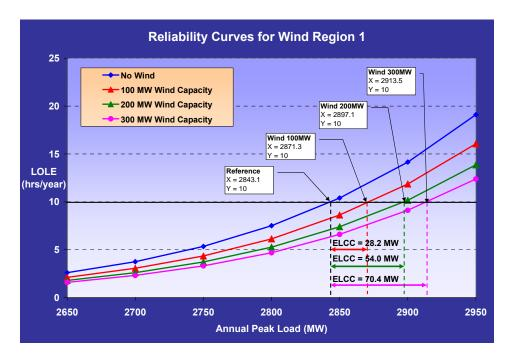
Figure 5-1: Region 1 capacity credit evaluation using reliability curves
