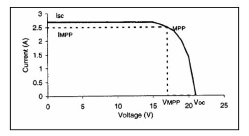
Figure 2-11: PV Cell Current-Voltage characteristics curve
