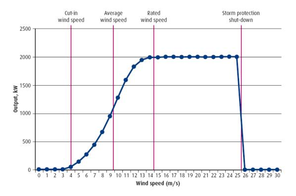
Figure 2-7: Wind turbine power curve (Source: Winkelman, 1992)
