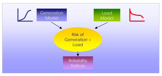
**Figure 2-1: Elements of generation reliability evaluation**
