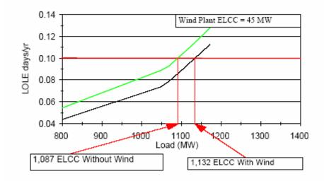
Figure 2-10: Reliability curves for calculating ELCC of a wind plant (Chen, pp. 89)
