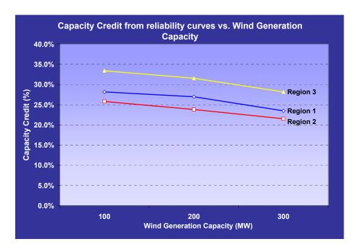
Figure 5-4: Capacity credit with different wind generation capacity
