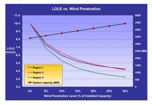
Figure 6-1: The effect of wind penetration on system reliability
