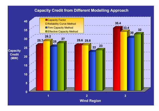
Figure 7-1: Capacity credit from different modelling approach
