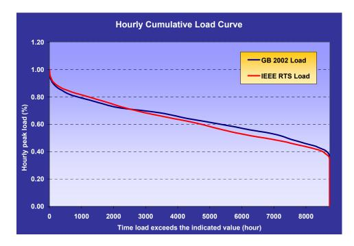
Figure 6-8: Hourly load duration curve comparison
