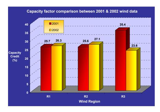
Figure 6-4: Capacity factor of wind generation capacity data for 2001 and 2002
