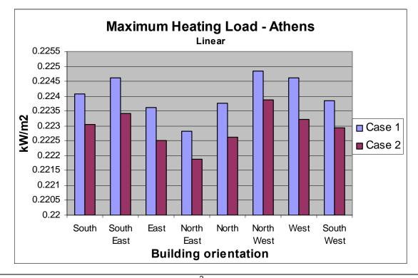
Figure 10: Maximum heating load per  $m^2$  - Athens
