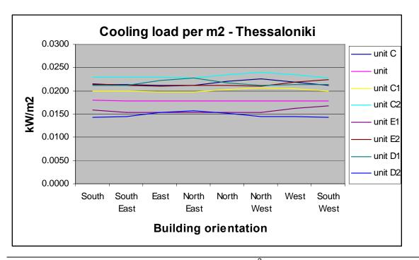
Figure 36: Maximum cooling load per zone per m<sup>2</sup> - Thessaloniki
