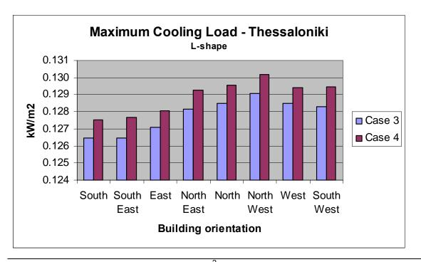
Figure 35: Maximum cooling load per m<sup>2</sup> - Thessaloniki
