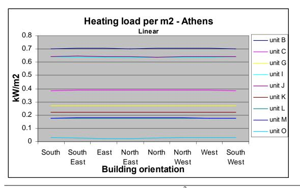
Figure 11: Maximum heating load per zone per  $m^2$  – Athens
