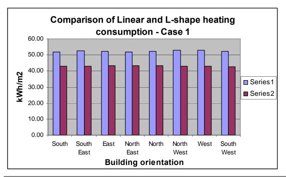
Figure 5: Heating consumption comparison – Athens – Case 1
