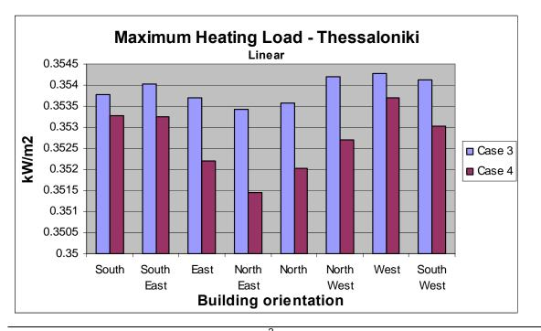
Figure 18: Maximum heating load per m<sup>2</sup> - Thessaloniki
