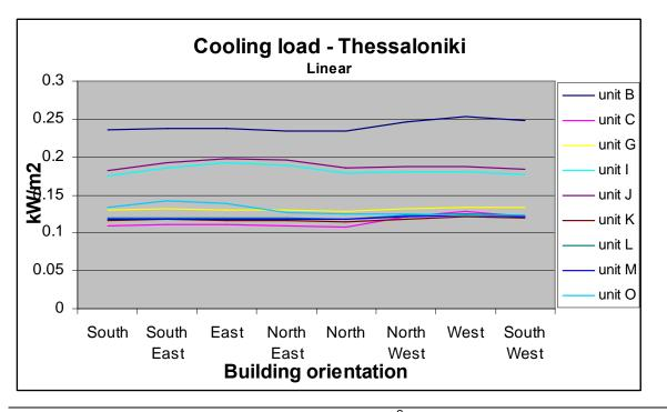
Figure 20: Maximum cooling load per zone per m<sup>2</sup> - Thessaloniki
