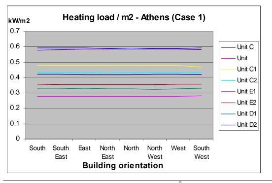
Figure 27: Maximum heating load per zone per  $m^2$  – Athens
