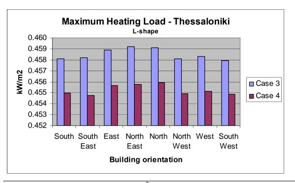
Figure 34: Maximum heating load per m<sup>2</sup> - Thessaloniki
