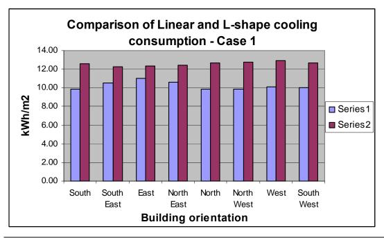
Figure 6: Cooling consumption comparison – Athens – Case 1
