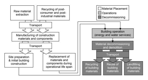
Figure 2.1: New building's life cycle assessment diagram
