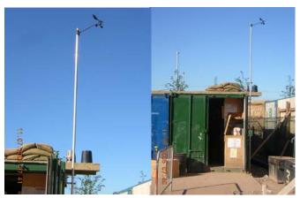
of momentum. The anemometer rotates proportionally to the speed of the prevailing wind to generate a signal. These signals are picked up by an electronic data logger. Typically cup anemometers have accuracy values of about  $\pm 2\%$ . Their
