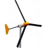
Almost all small horizontal axis wind turbines use a tail vane to direct it into the wind. Tail vanes are used instead of yaw motors and mechanical drives whose sizes cannot be accommodated in the small wind turbines. Figure 2.4 shows a typical three bladed small wind turbine with a tail vane.
