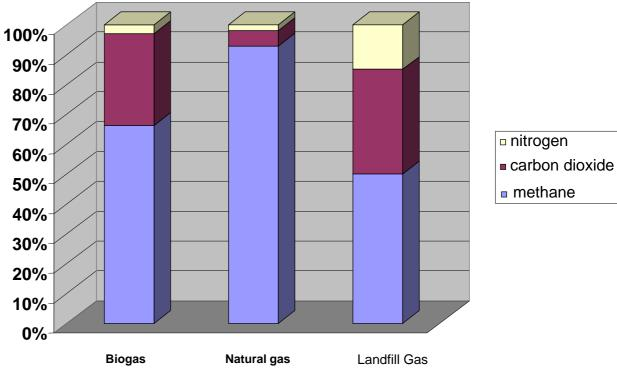
figure 8. Composition of different gases.
