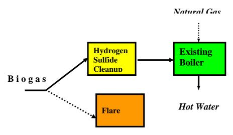
figure 21. Case1-Hydrogen Sulphide Removal
