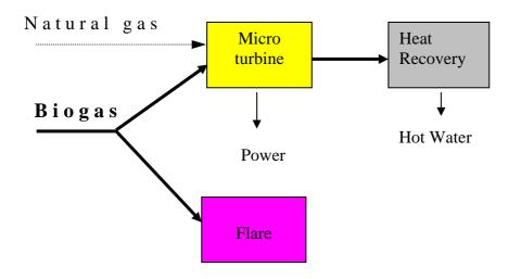
figure 18. Case 2: Microturbine With heat Recovery
